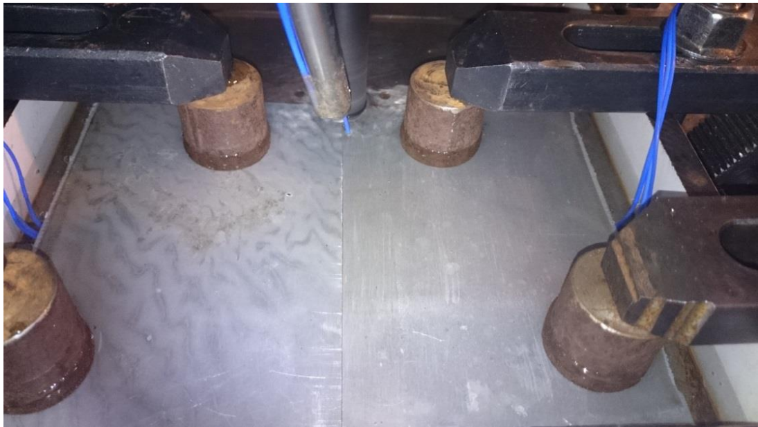
Figure 4: WC FSW Setup
