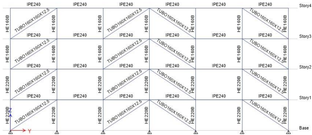
Figure A62: Design Section 4-Story H Plan Concentric Diagonal Braced Frame External Section on Y-axis
