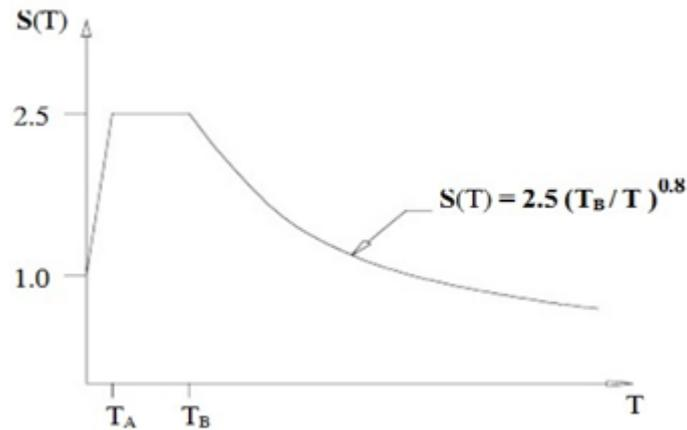
Figure 2.1. Design Acceleration Spectrums [9].
