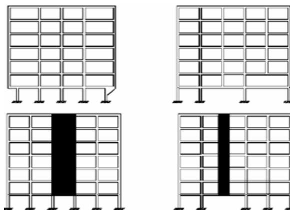
Figure 4.8. Type B3- Discontinuities of Vertical Structural Elements [9].
