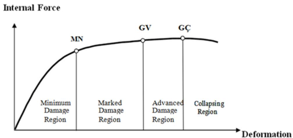
Figure 2.2. Member damage levels and member performance regions on capacity curve [9].
