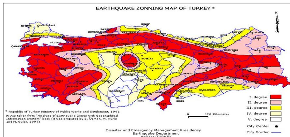
Figure 4.10. Seismic Hazard Zonation Map of Turkey [35].
