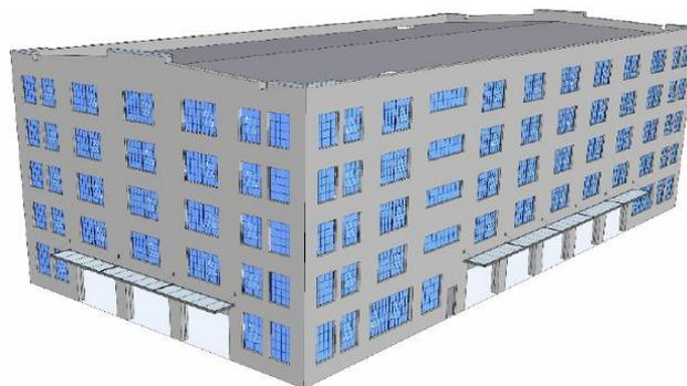
Figure 4.6. Illustration of a building with a soft ground story due to large openings and narrow piers.
