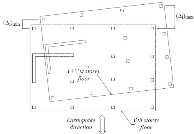
Figure 4.2. Type A1- Torsional Irregularity [9].
