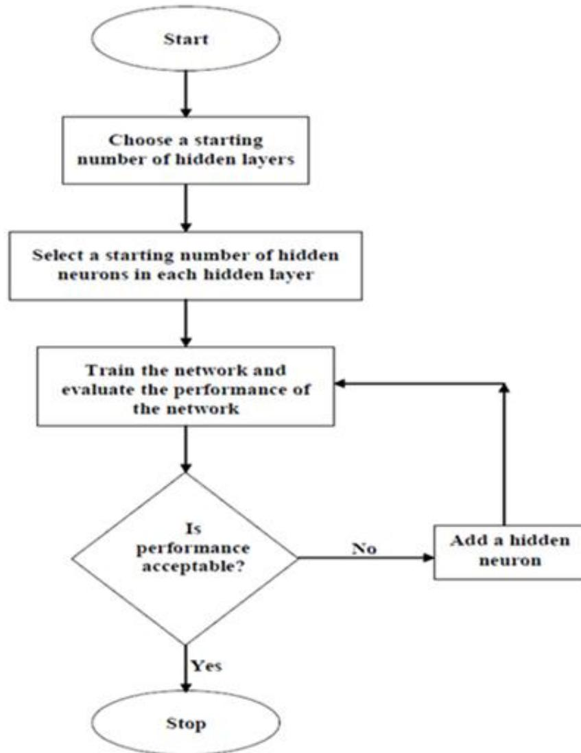
Figure 4.11. Flow chart for training process of neural networks [32]
