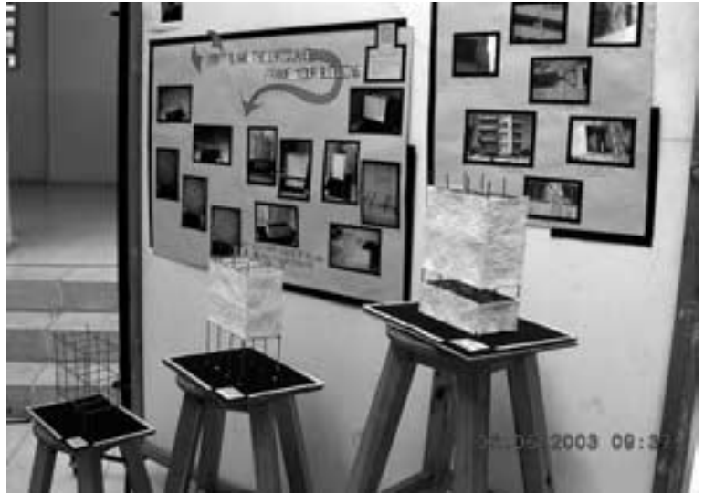
Figure 5. Abstract models, which represent the formation of soft storey and short column problems, and the students' poster.
