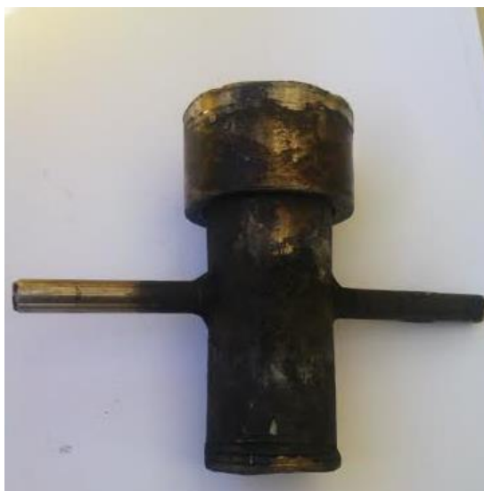
Figure 63. Cylindrical receiver-tube used in solar torrefaction process.
