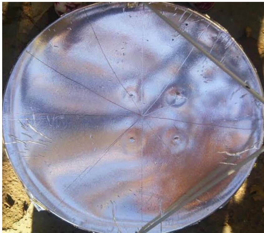
Figure 62. Parabolic dish antenna covered by reflective material for concentration of solar thermal energy.
