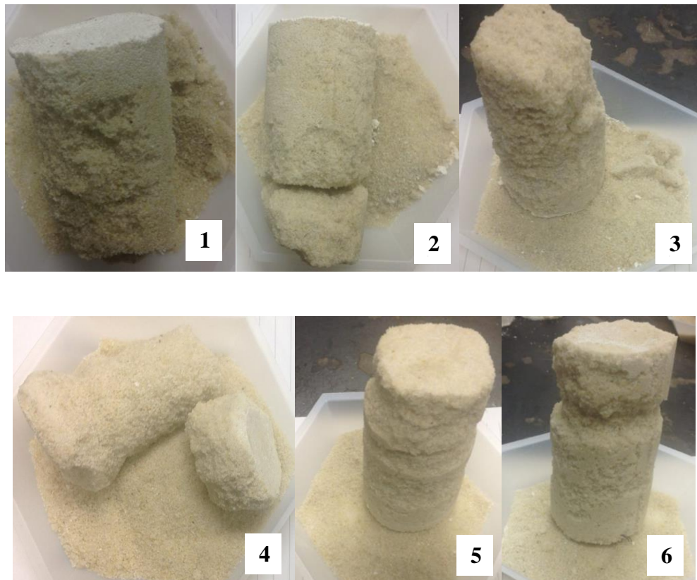
Figure 6.18. Treated samples by using soaking method at the lowest rate.
