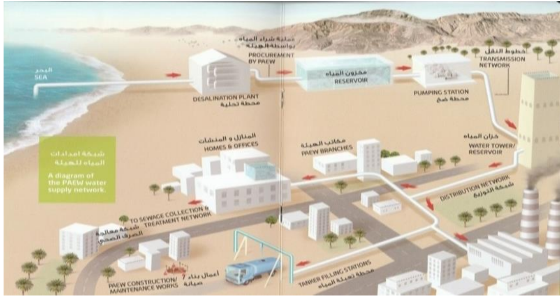
Illustration 1: A diagram of the PAEW water supply
