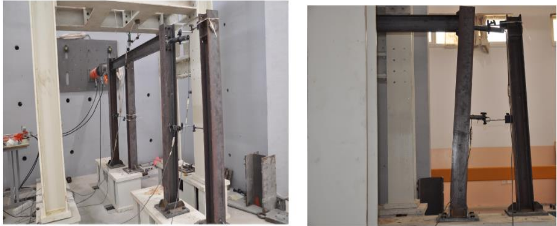
Figure 3.13: Experimental specimen MIN-1B-1S before and after the test [11].
