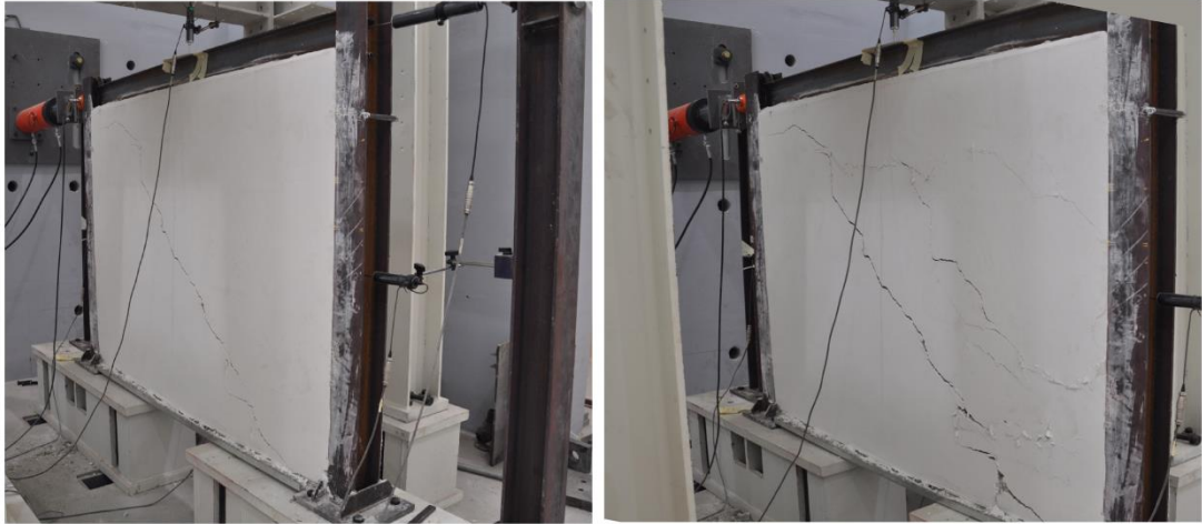
Figure 3.16: The formation of diagonal and hairline cracks [11].
