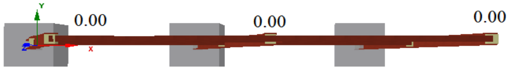
Figure 4.24: Plan view of minor axis 2 bay 2 story (2B-2S) models illustrating out-of-plane displacements at node 1-3.
