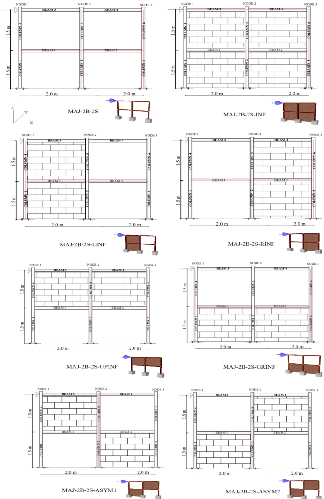
Figure 4.9: Details of major axis 2 bay 2 story (2B-2S) models with SeismoStruct illustrations.
