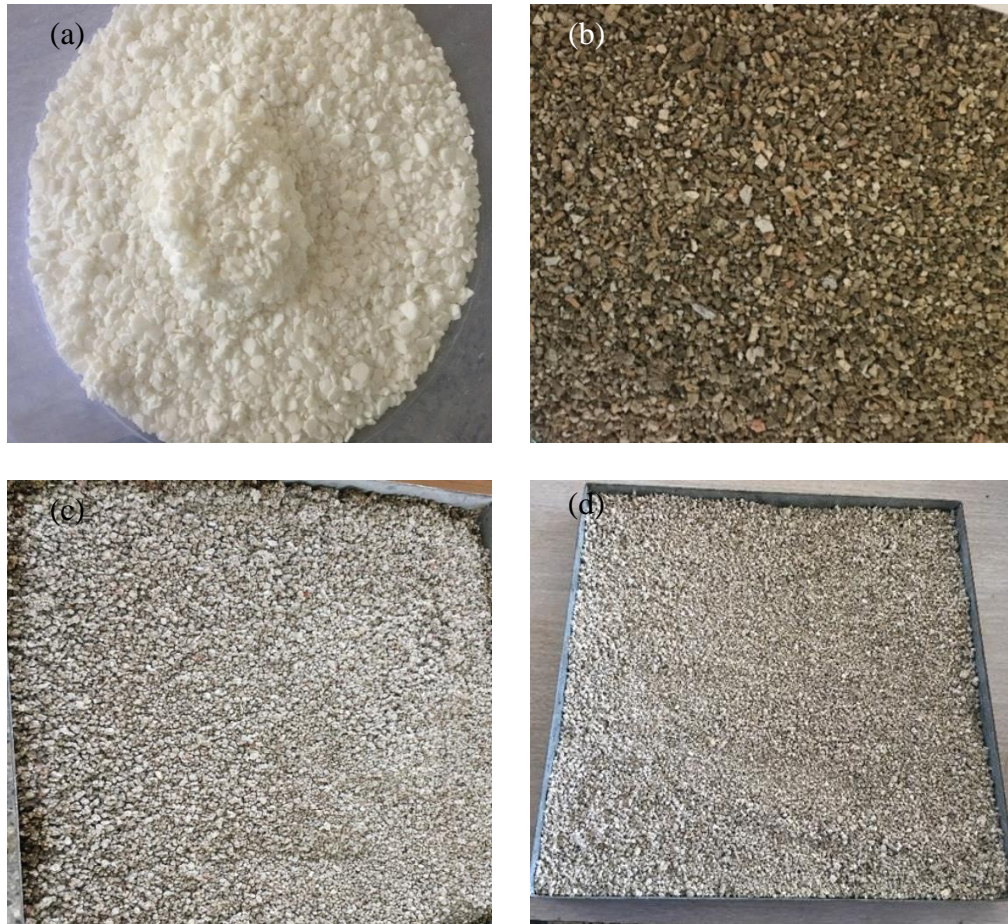
Figure 8: (a) Anhydrous \text{CaCl}_2 , (b) Vermiculite, (c) V- \text{CaCl}_2 After Charging (not well dried), (d) V- \text{CaCl}_2 After Charging (well dried)
