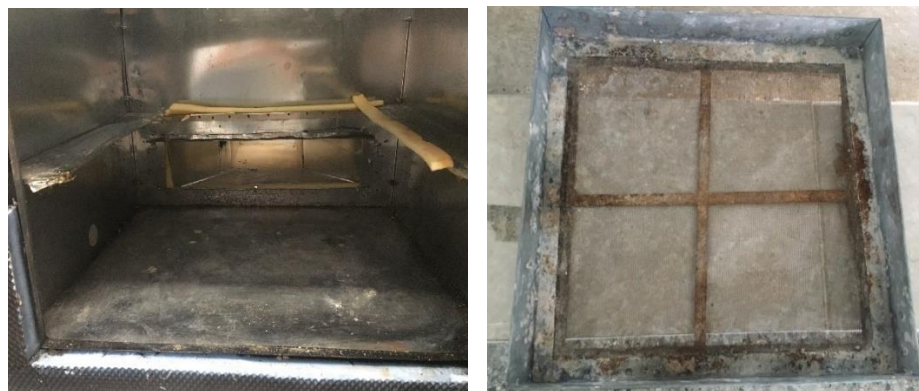
Figure 12: (a) Internal View of Sorption Reactor, (b) Perforated Tray
