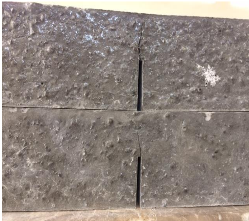
Figure 5.16: Failure Mode of Notched Flexural Specimens
