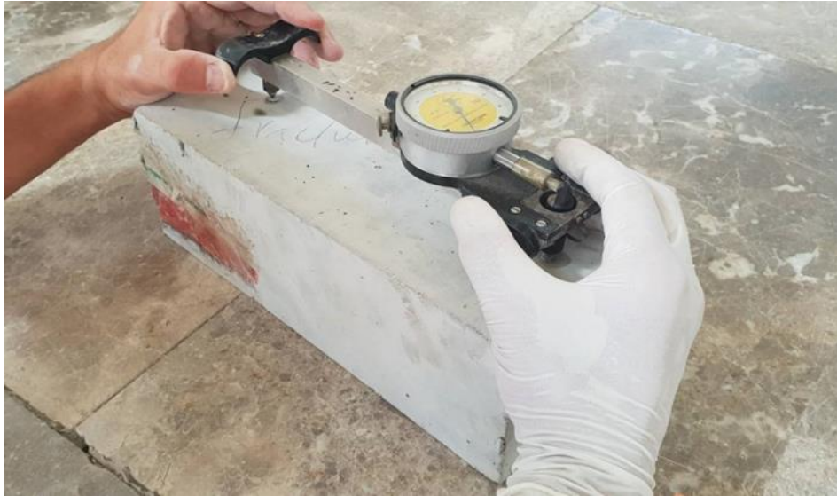
Figure 13: Measuring the displacement between the pins using the apparatus
