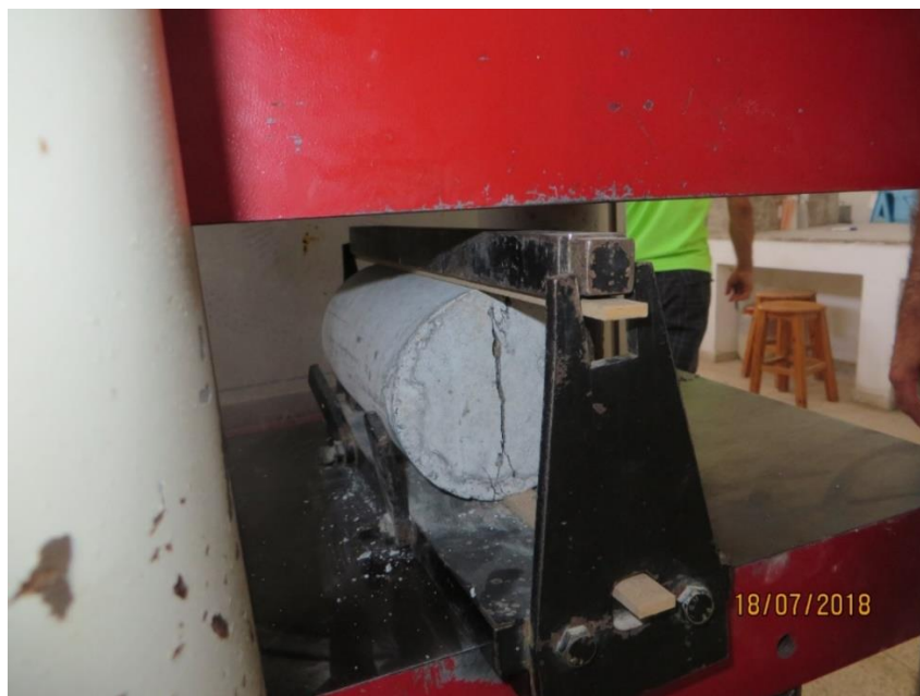
Figure 11: Specimen failure under stress (splitting tensile)
