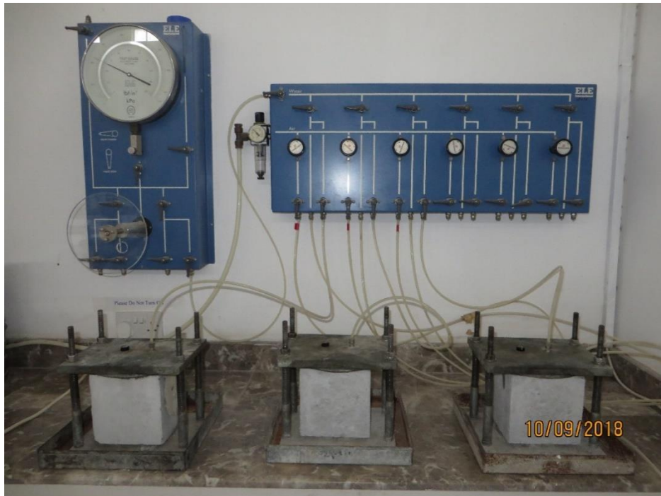
Figure 16: Water penetration test apparatus
