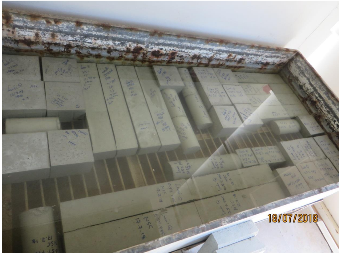
Figure 8: Curing specimens in water tank
