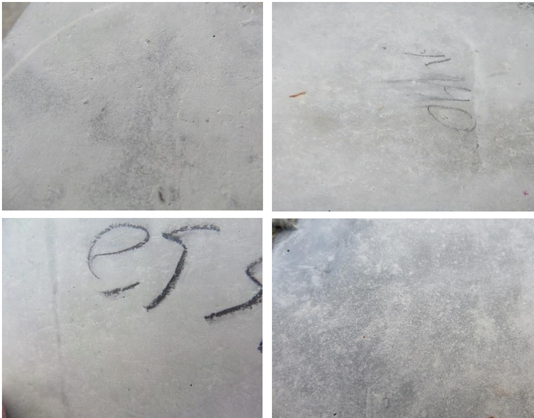
Figure 43: Surfaces of PPF specimens after heating
