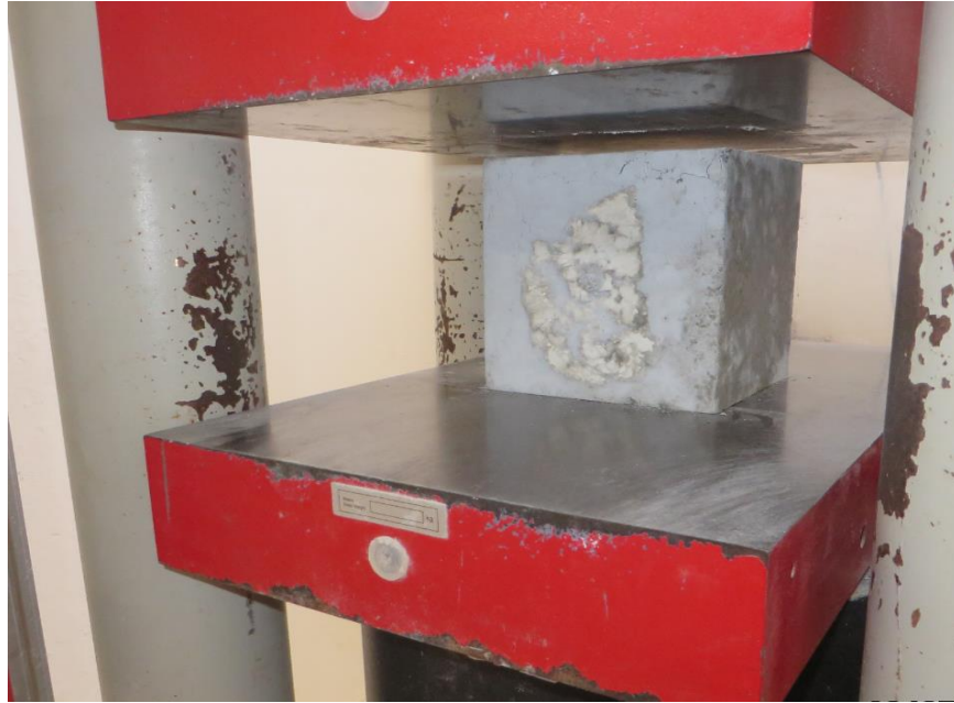
Figure 9: Specimen failure in compressive strength test
