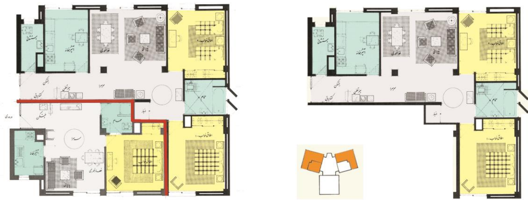
Figure 27. The combination of one bedroom and two bedroom units. Source: Ali Adibi Consulting Engineering Company.
