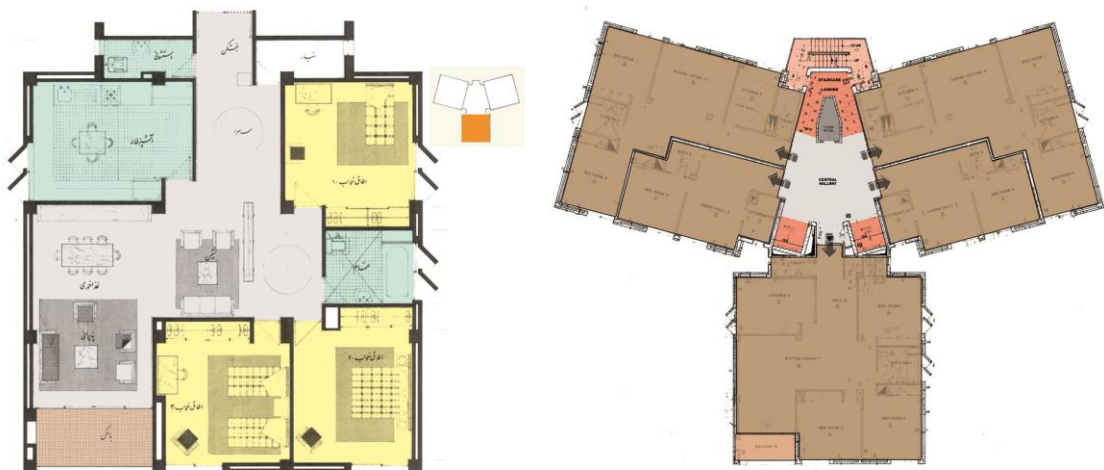
Figure 28. Three-bedroom unit (left) and Typical Floor Plan (right). Source: Ali Adibi Consulting Engineering Company.
