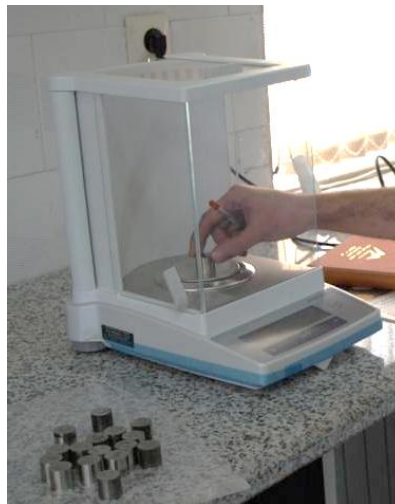
Figure 3.3: Balancing Machine with accuracy equal to 0.00001 gram
