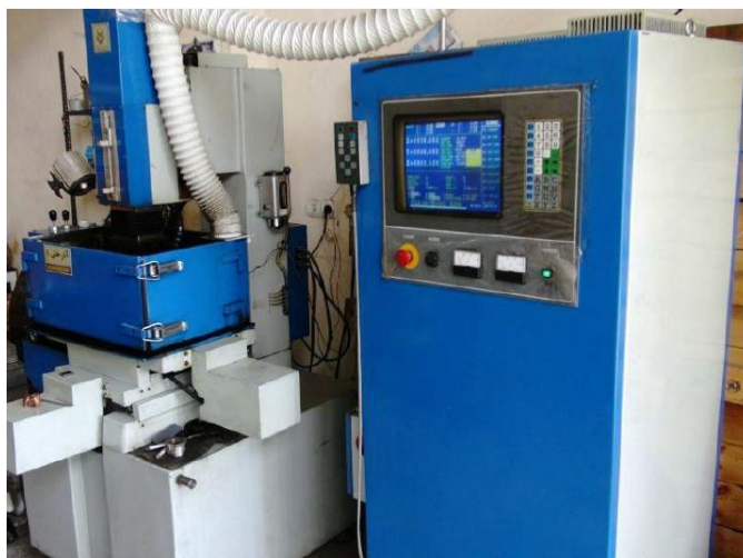
Figure 3.2: Electrical Discharge Machining
