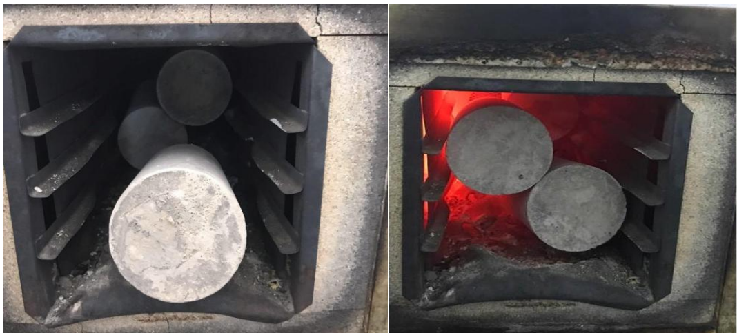
Figure 3.7: Heating Samples to Test Heat Resistance Testing of Concrete with Different amount of QP
