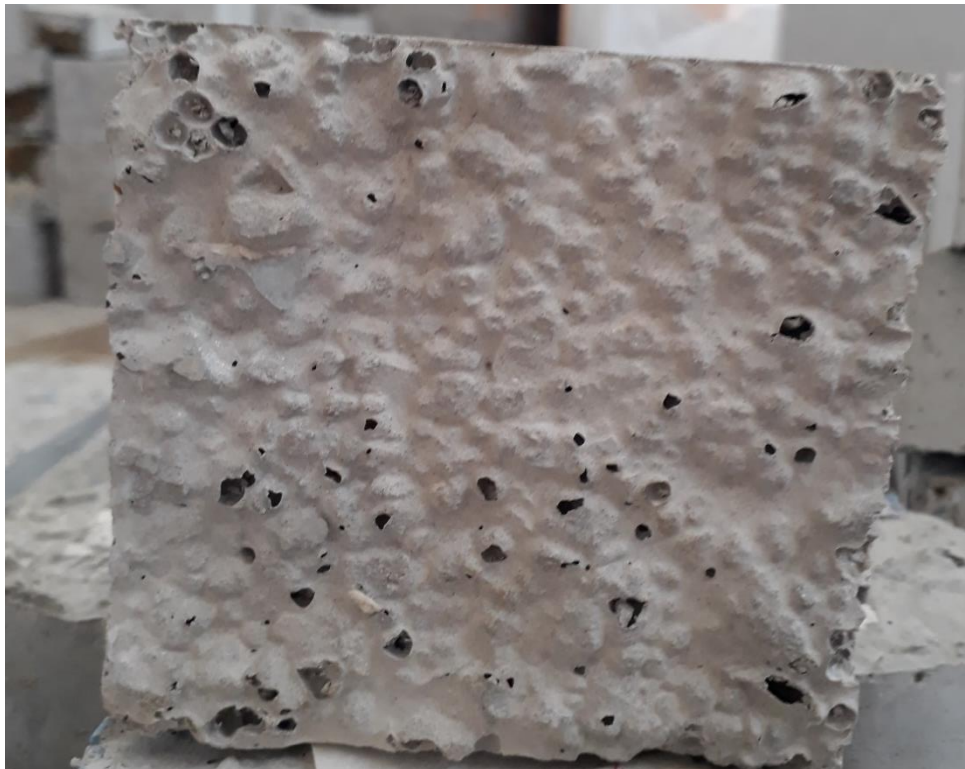
Figure 4.19: PS-SCC Specimen after Heat Exposure at 200 °C
