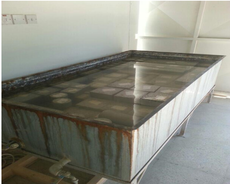
Figure 3.9: Water Curing of Concrete Specimens
