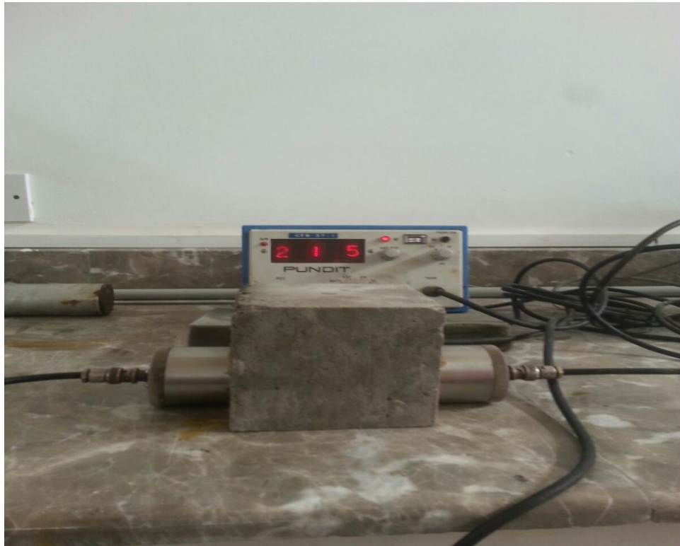
Figure 3.12: Ultrasonic Pulse Velocity Test (UPV) Device
