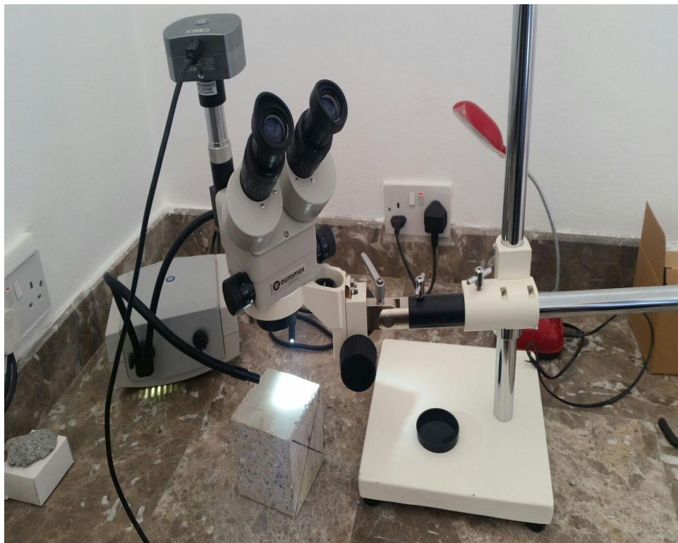
Figure 3. 14: Investigating Cracks on the Surface of Specimens by Using Stereo-Microscope
