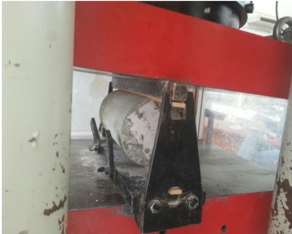
Figure 3.11: Splitting Tensile Strength Testing Device
