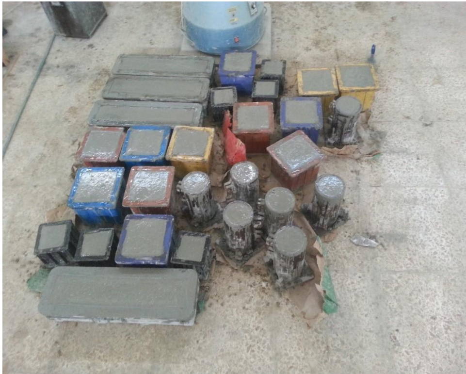
Figure 3.8: Cylindrical, Cubic and Beams Test Specimens
