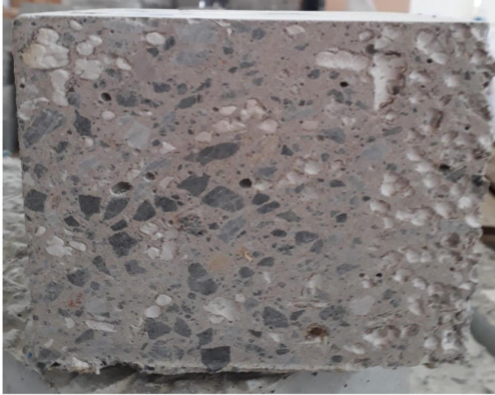
Figure 4.18: PS-SCC Specimen after Heat Exposure at 100 °C
