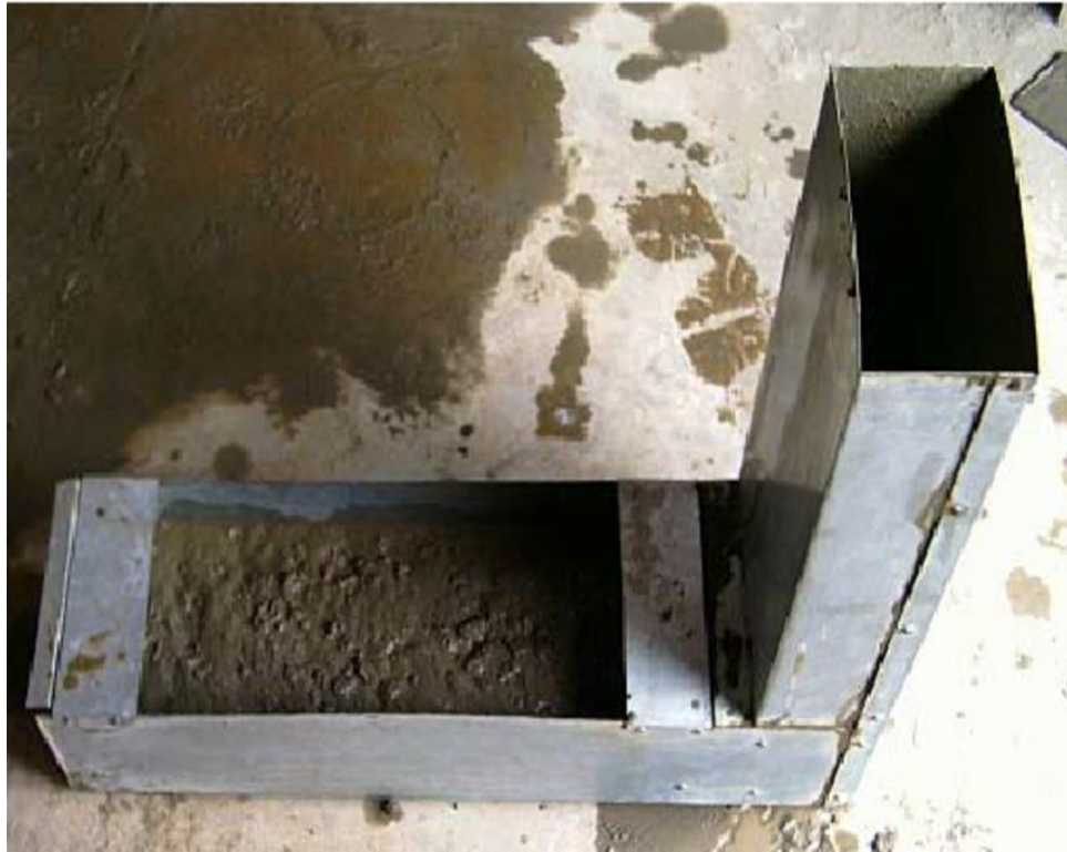
Figure 3.7: L-Box Testing Equipment
