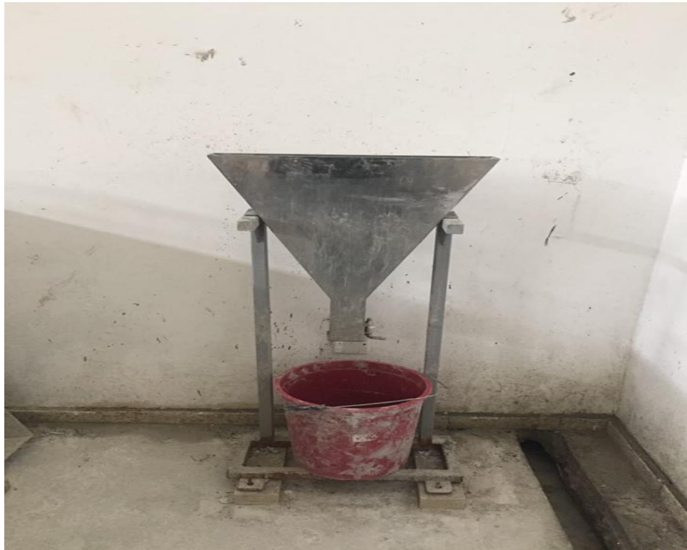
Figure 3.6: V-Funnel Testing Equipment
