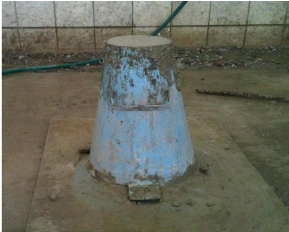
Figure 3.5: Concrete Slump Test
