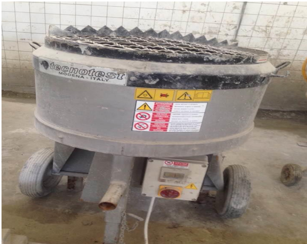
Figure 3.8: Concrete Mixer of 0.25 m 3 Capacity
