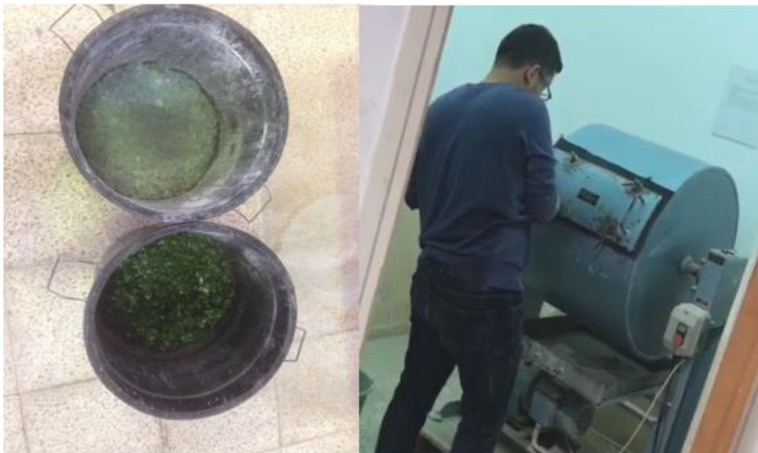
Figure 3.4: Crushing of Waste Glass to Coarse and Fine Aggregate Sizes
