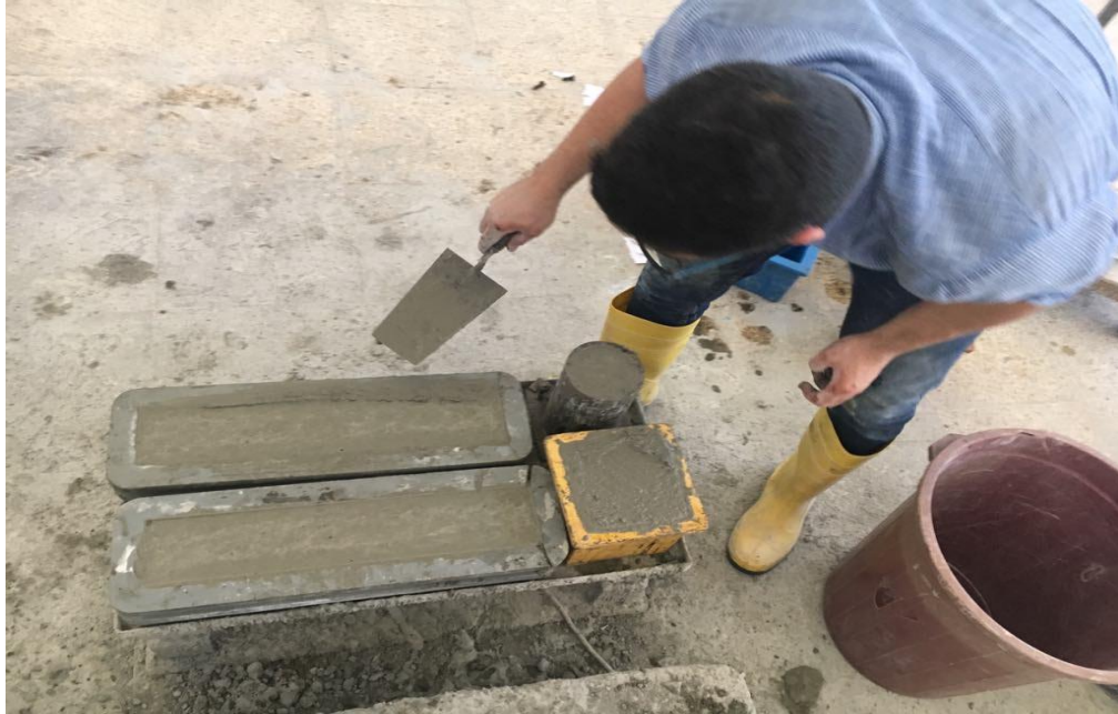
Figure 3.10: Standard Compaction of Specimens
