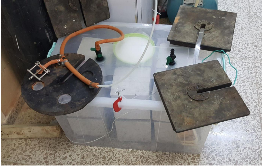
Figure 3.15: The Carbonation Chamber
