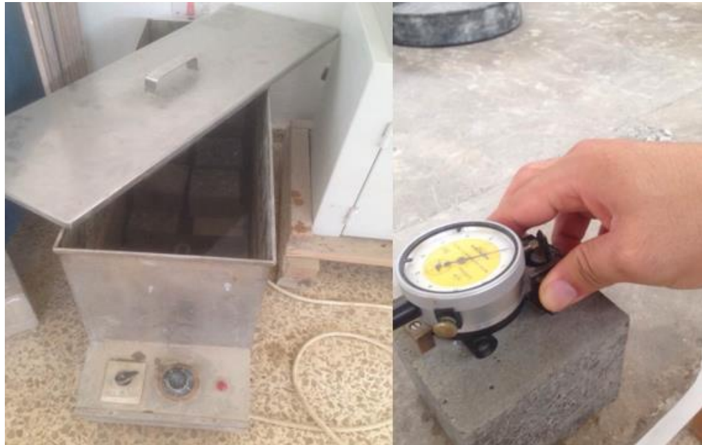
Figure 3.16: Water Bath & DEMEC Gauge
