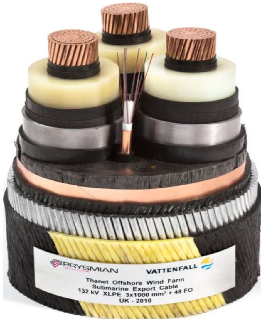
Figure 2.30: Three-phase copper core HVAC submarine power cable (132 kV) together with fiber optic, Prysmian manufacture
