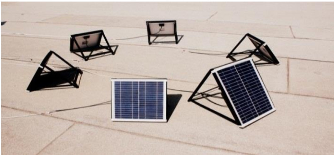
Figure 3.15: Arrangement of 6 PV Modules with Different Orientations for Output Power Data Collection
