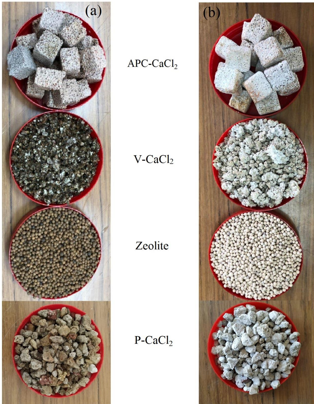
Figure 18: Images showing the tested materials after discharging (a) and after charging (b)
