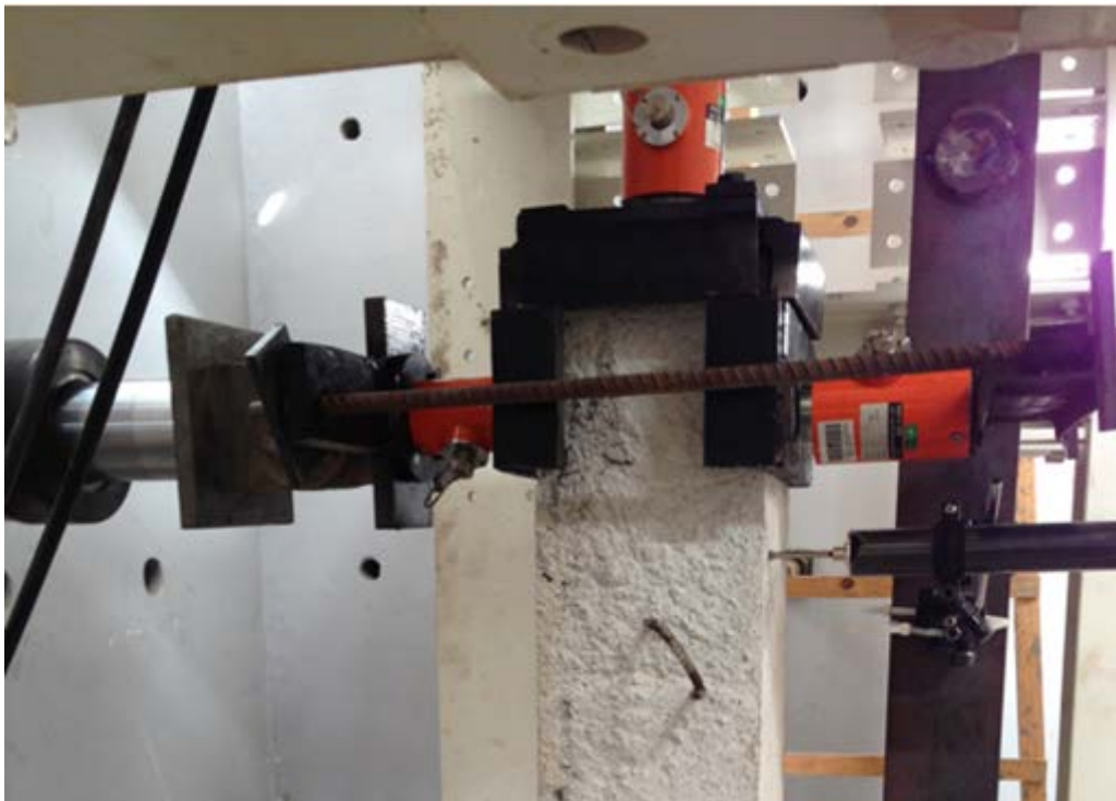
Figure 3.7. Details of hydraulic jacks and load cells placement
