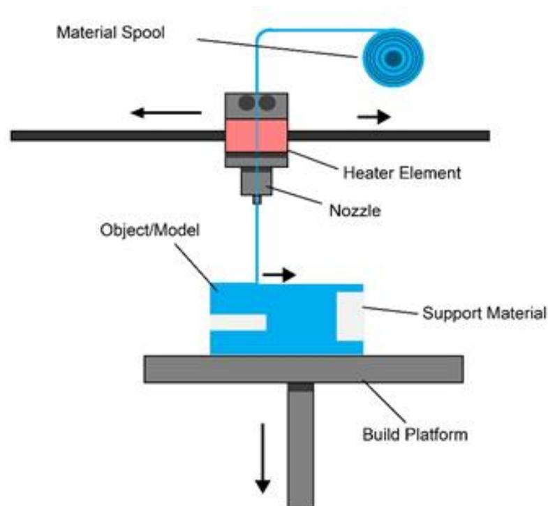
Figure 4: Material Extrusion (URL 2)
