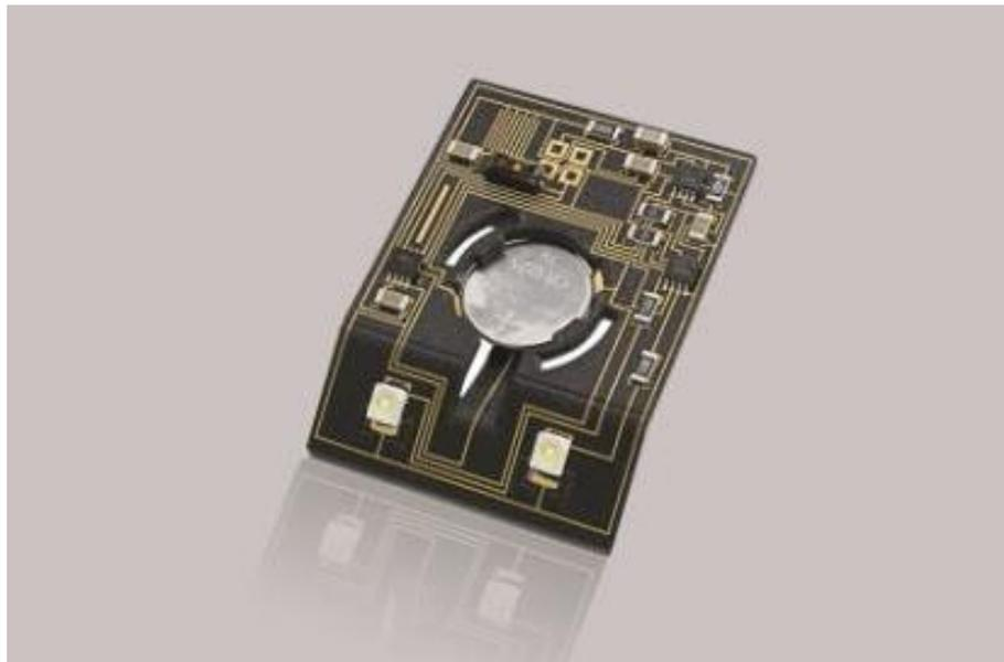
Figure 14: 3D Printed Circuit Board (URL 8)
