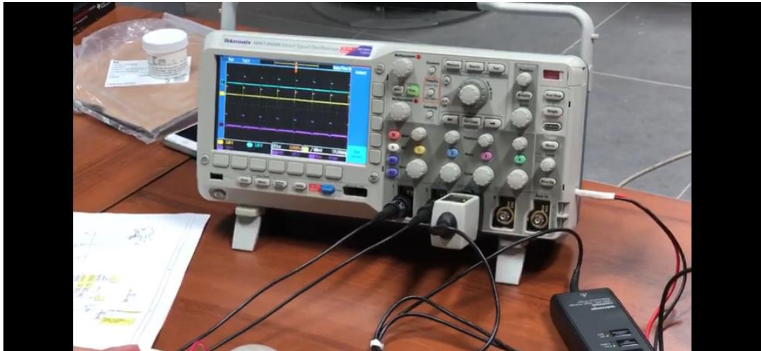
Figure 51. Tektronix oscilloscope to monitor the voltage and current.
