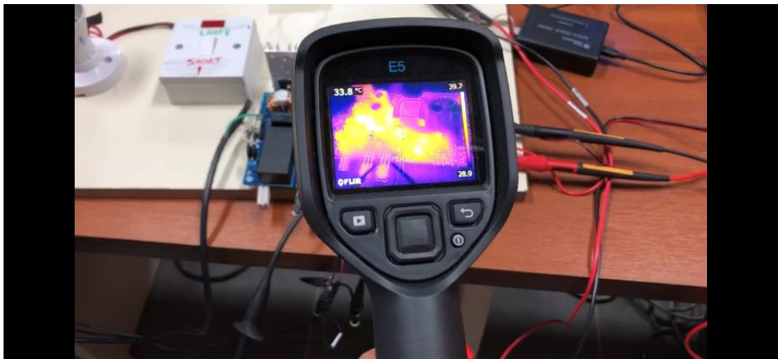
Figure 50. Thermal camera used to monitor the components temperature.
