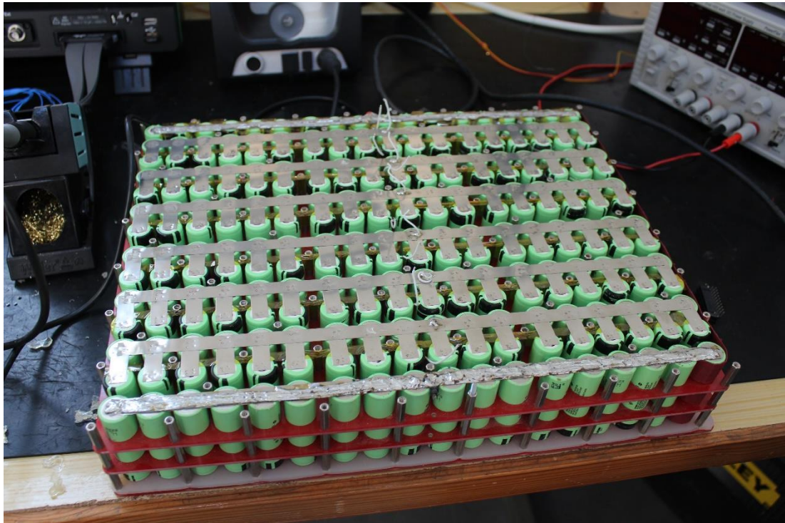
Figure 47. NCR18650B Panasonic batteries that used in the experiments.
