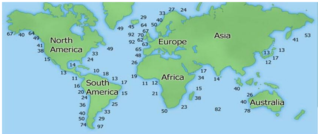
Figure 1.1: The relative strength of wave energy in kW/m observed all around the world. ( URL:1 ).
