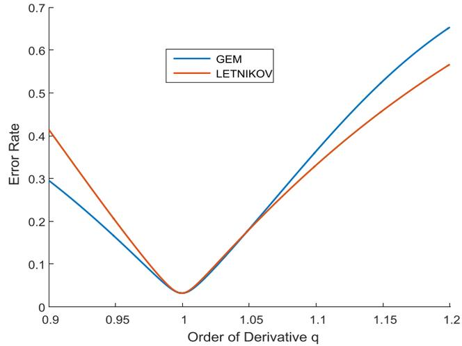
Figure 4.2: PSE and GEM error rate (MSE%) versus possible  $q$  values.
