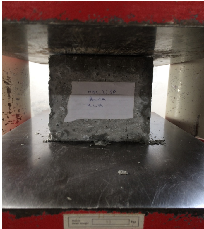
Figure 10: Specimen failure in compressive strength
