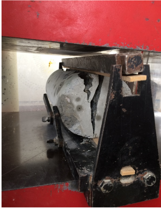
Figure 12: Specimen failure in splitting tensile strength
