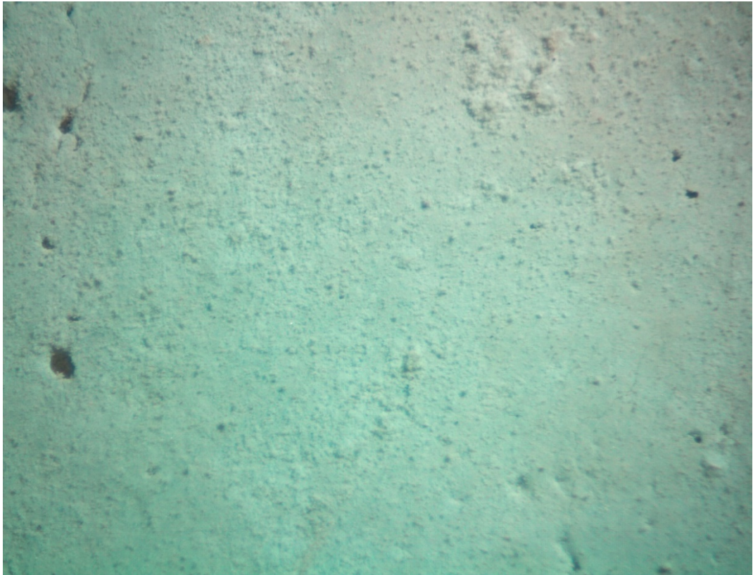
Figure 44a: NSC-control mix surfaces after 200 °C heating at 28 days
