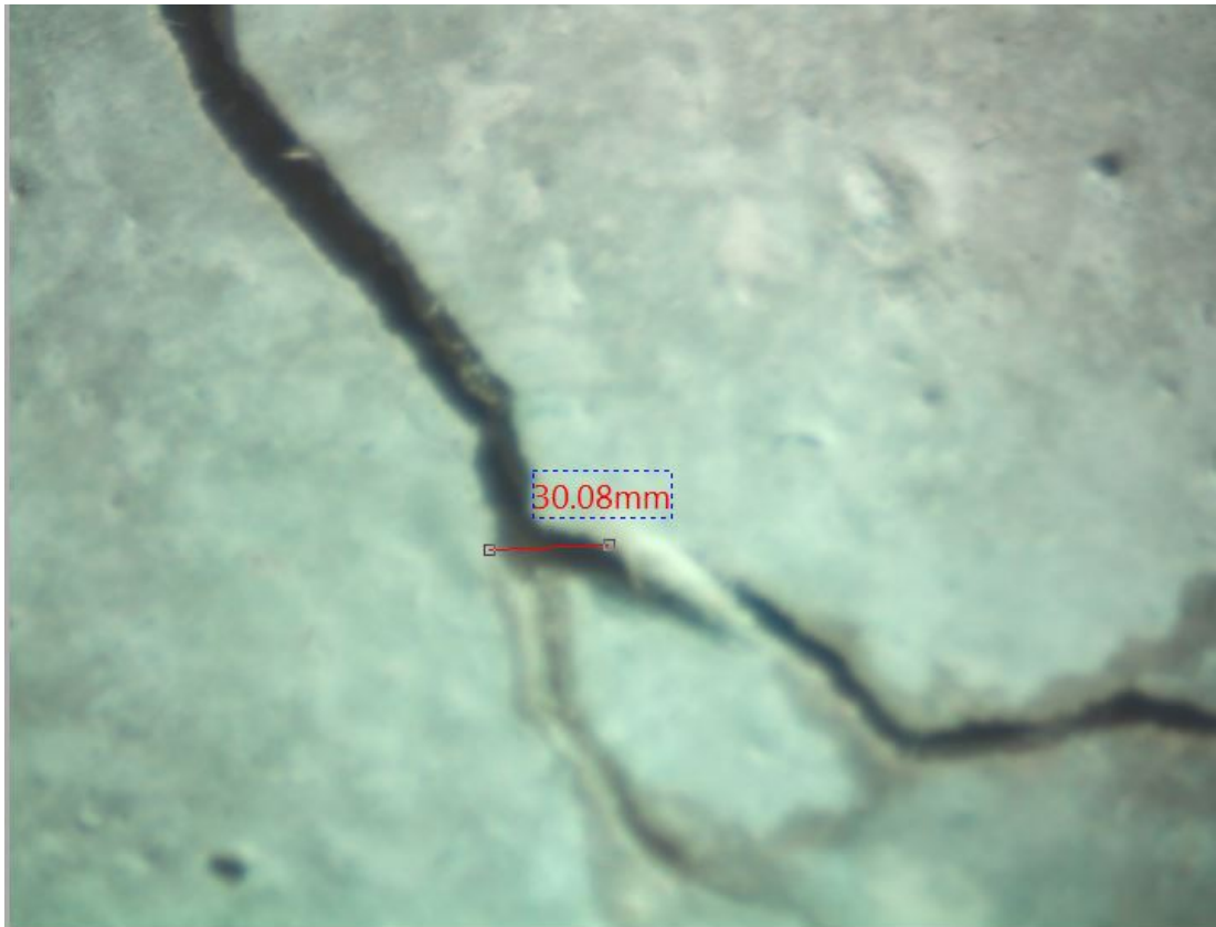
Figure 46f: HSC-50% PP surfaces after 200 °C heating at 28 days
