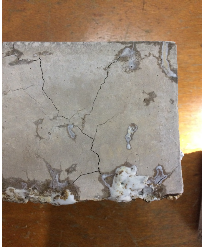
Figure 16: Crack development of sample after heat exposed
