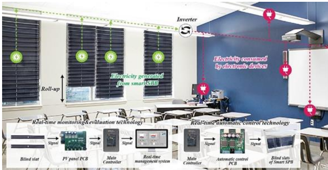
Figure 20: Real-time tracking, analyzing and automated management of the smart SPB, (Kang et al., 2019)
