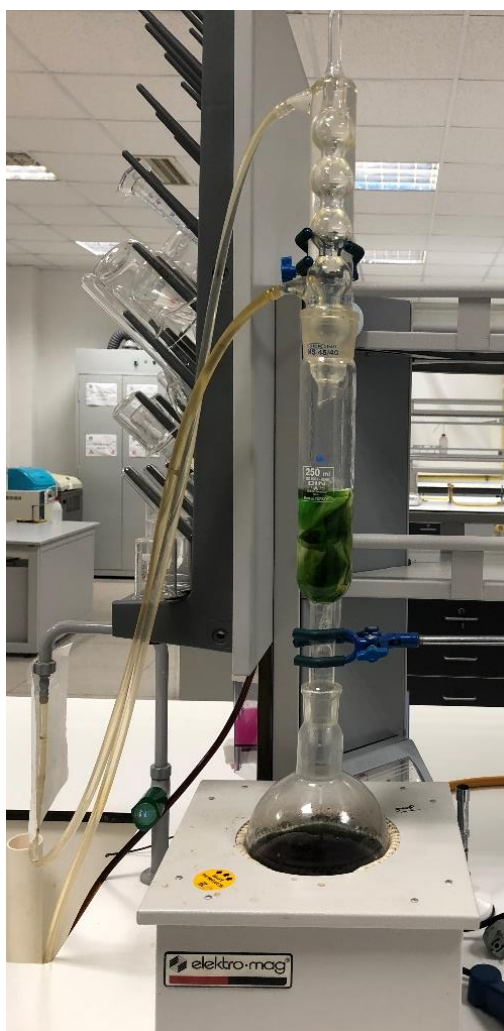
Figure 7: Extraction of Corchorus olitorius L. by Using the Soxhlet Equipment
