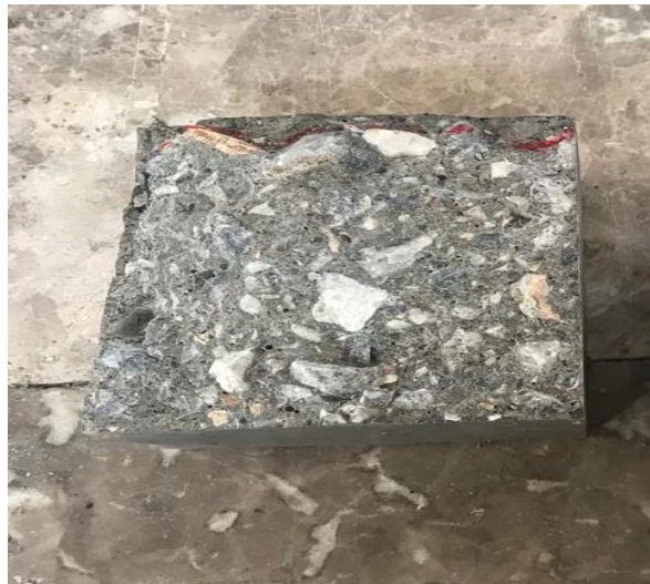
Figure 4.8: Marked Depth of Water
