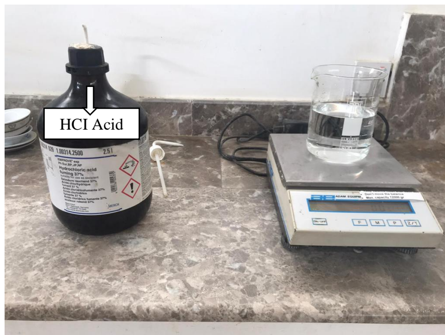
Figure 4.14: HCl Acid Used for Cleaning the Corroded Steel Bars
