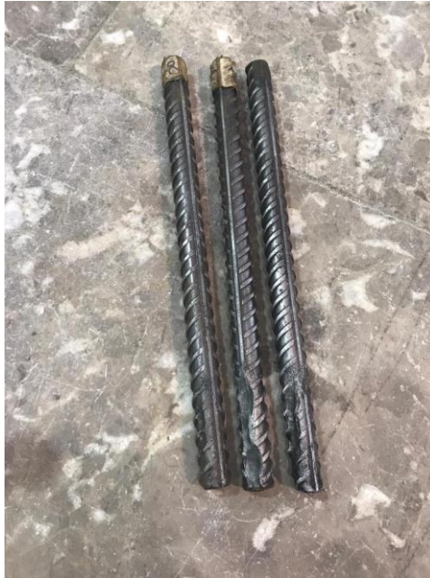
Figure 4.15: Cleaned Steel Bars after HCl Acid Wash
