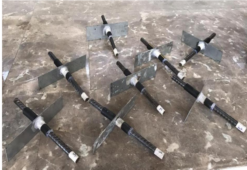
Figure 4.12: Designed Formwork of Steel Bars
