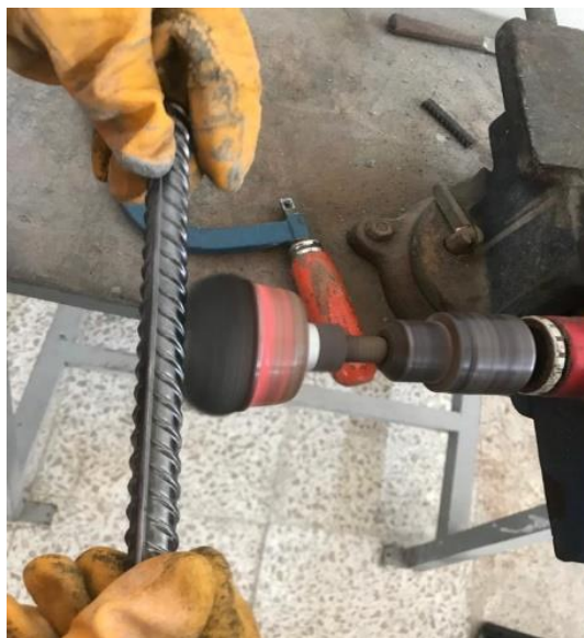
Figure 4.11: Brushing Process of the Steel Bars
