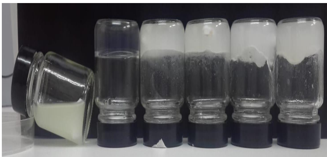
Figure 18: Hydrogel Formation with Different Ratios of Vinyltrichlorosilane Chitosan/Acrylamide Combination. Molar Ratio of Acrylamide Increases from Left to Right 0:1, 1:3, 1:5, 1:7 and 1:9.
