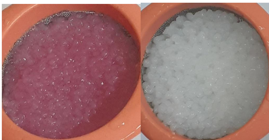
Figure 3.1: Co(II)-I beads formed before and after removal of the cobalt template.
