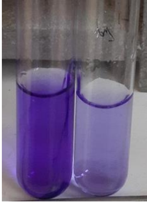
Figure 4.20: Crystal violet dye solution (20 mg/L) before and after adsorption.
