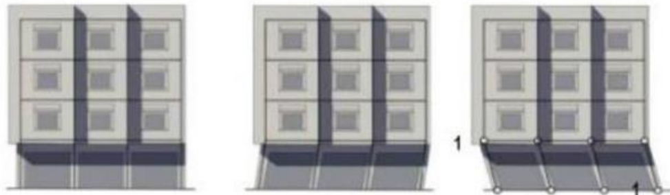
Figure 14: Model of plastic hinges at the junction of soft story and other floors[39]
