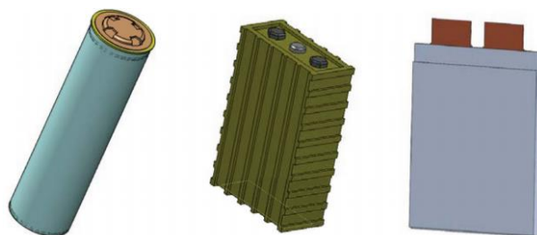
Figure 1: Lithium Ion Cell Types [4]
