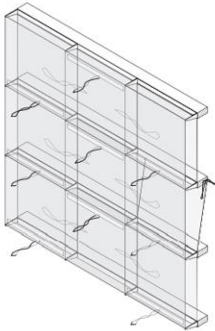
Figure 6: On Left Section of Shaft Box Façade, And on The Right ARAG Tower, Düsseldorf, RKW Architektur + Städtebau with Foster and Partners, 2000, (Knaack, U. et.al.,2007).
