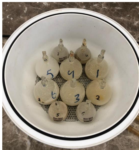
Figure 3.14: Pycnometers containing dried ground samples, approximately 10g and half fully with deionized water
