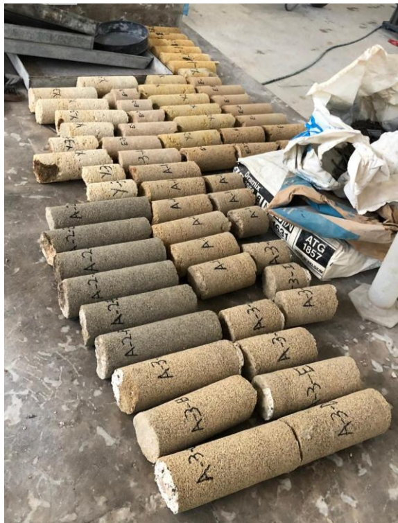
Figure 3.3: Removed samples from natural stones by coring machine
