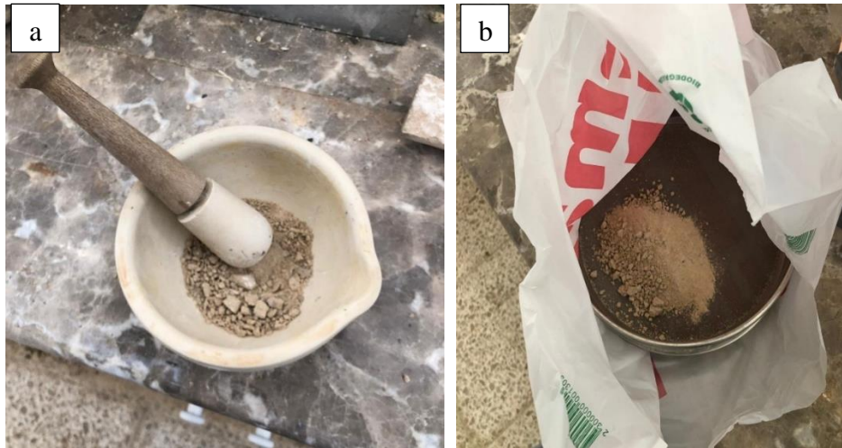
Figure 3.12: a) Grinding of samples and passing through sieve stage 1 b) Stage 2
