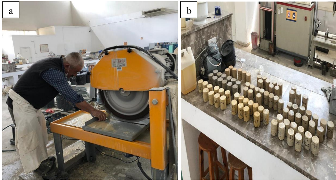
Figure 3.4: a) Cutting samples to approximately 64x64 mm cylindrical shape stage 1 b) Stage 2
