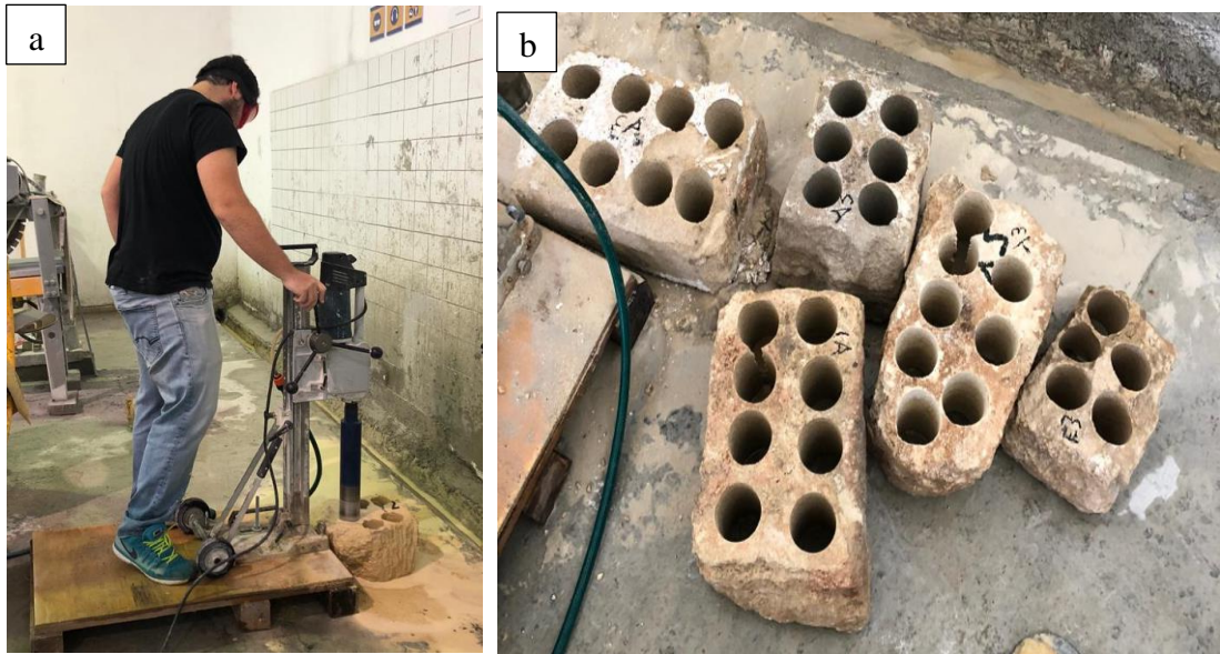
Figure 3.2: a) Removing of testing samples from natural stones stage 1 b) Stage 2
