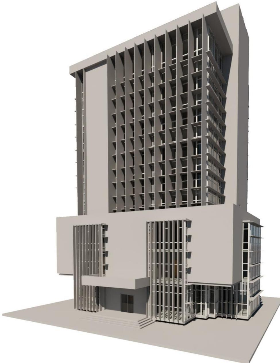
Figure 57: 3D View of Egg-Crate Shading System at the West Façade (Author, 2021)
