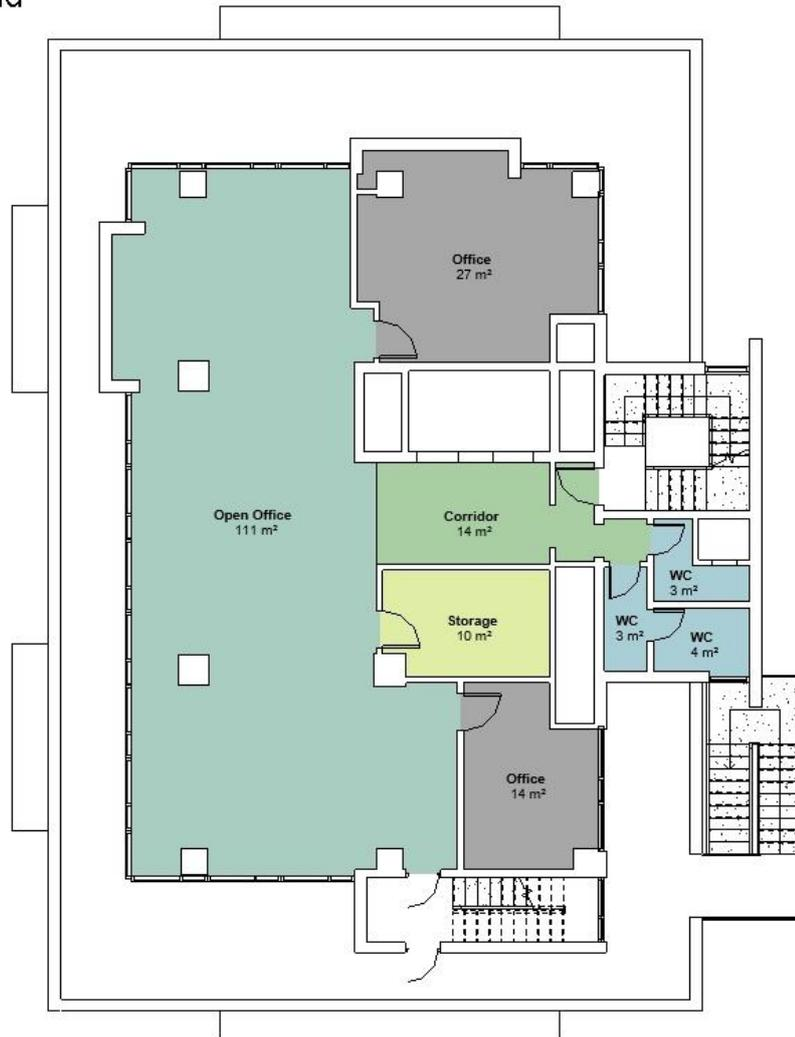
Figure 43: Level +11.81 Floor Plan of KPMG Building (Author, 2021)
