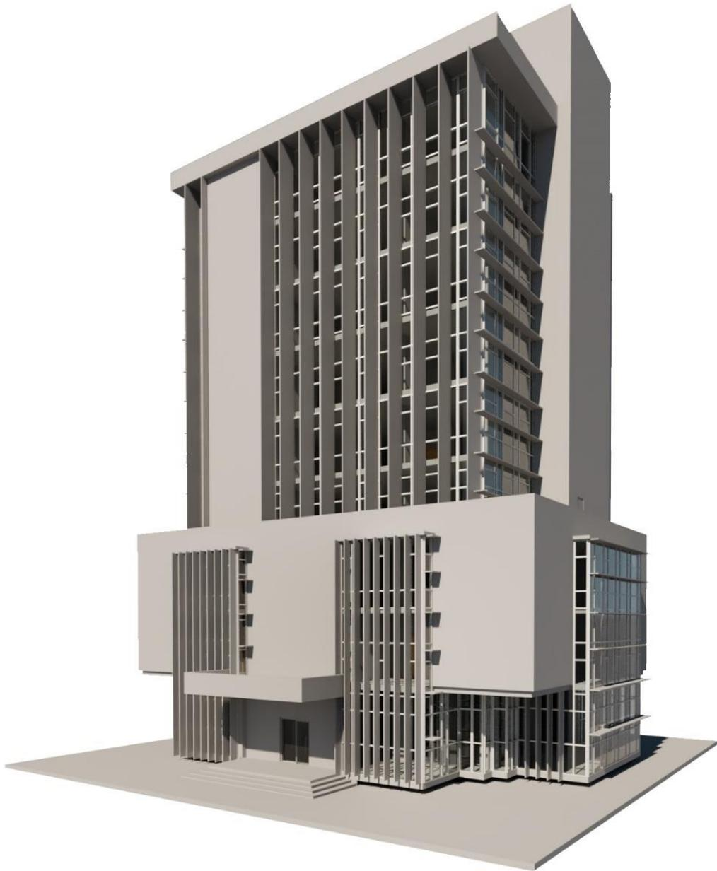
Figure 51: 3D View of the Louver and Fins system at the West and South Façade (Author, 2021)
