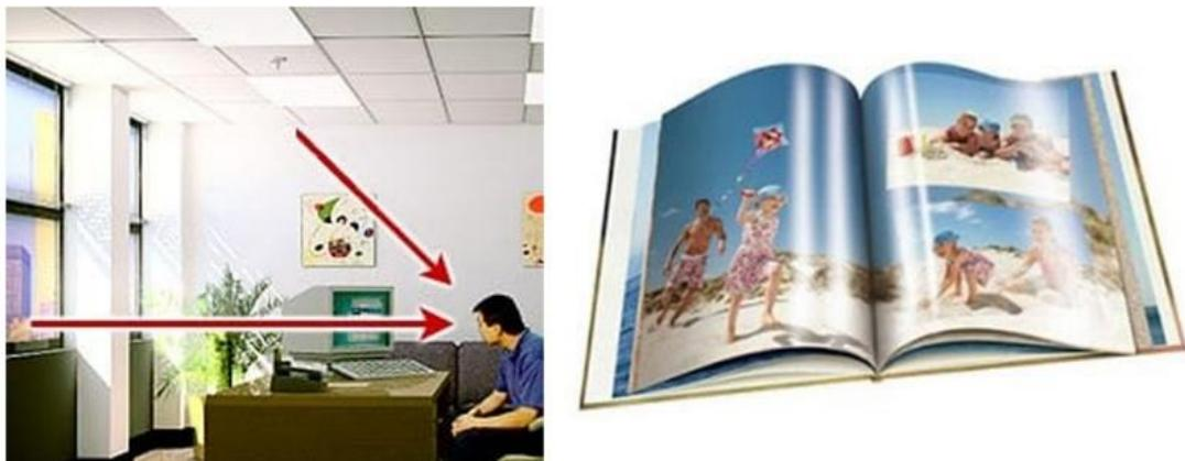
Figure 4: (Left to Right); Direct Glare, Veiling Reflection (URL, 3)
