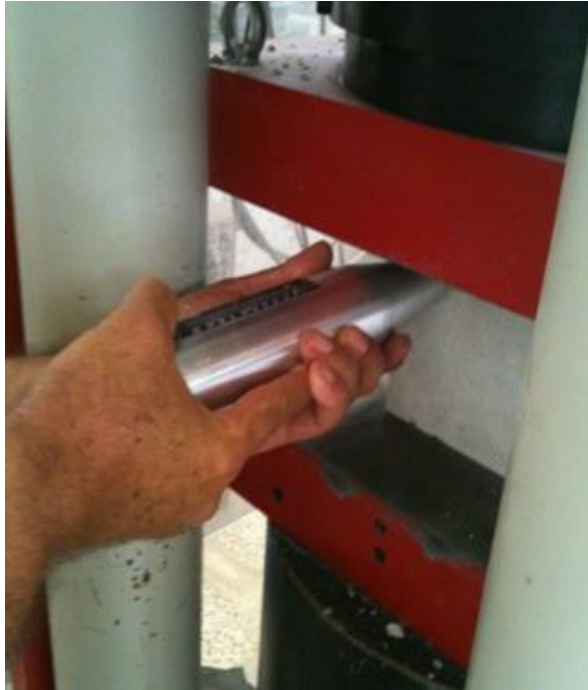
Figure 3.11: Rebound hammer test
