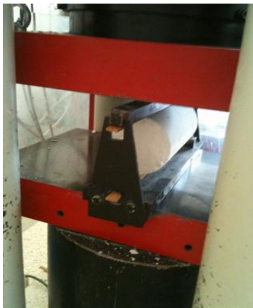
Figure 3.8: Cylinder specimen under splitting tension
