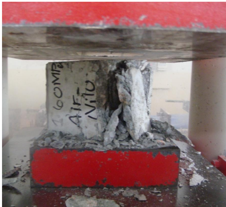
Figure 4.54: Fractured cubic specimen
