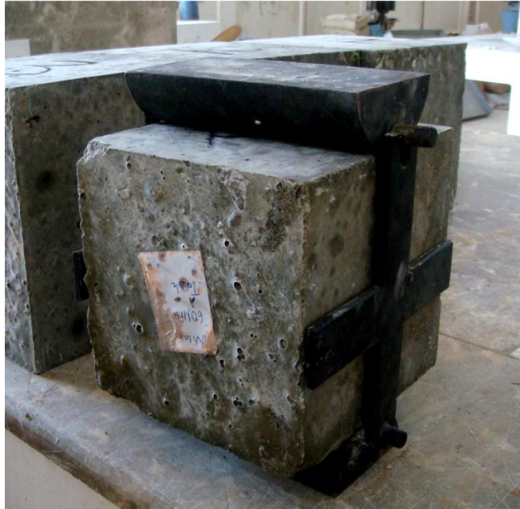
Figure 3.9: Cubic specimen setup before splitting tension
