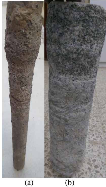
Figure 4.14: Hardened deformed shapes of the SCs a) NEC-EBSC with 5cm diameter b) NEC-EBSC with 10 cm diameter
