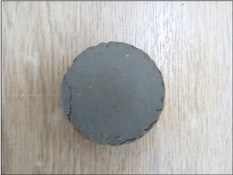
Figure A.27. Sample preparation of one dimensional consolidation test at 22.5% initial water content
