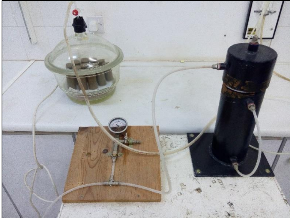
Figure 3.3. Vacuum drying setup
