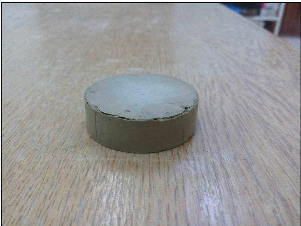
Figure A.28. Sample preparation of one dimensional consolidation test at 16% initial water content
