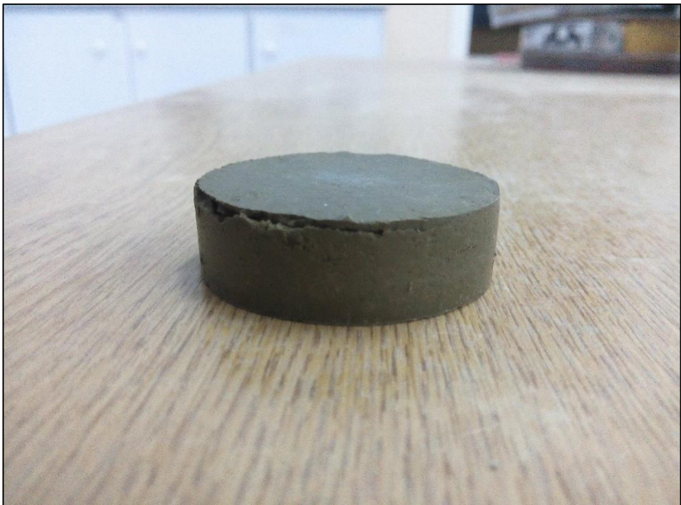
Figure A.26. Sample preparation of one dimensional consolidation test at 28% initial water content
