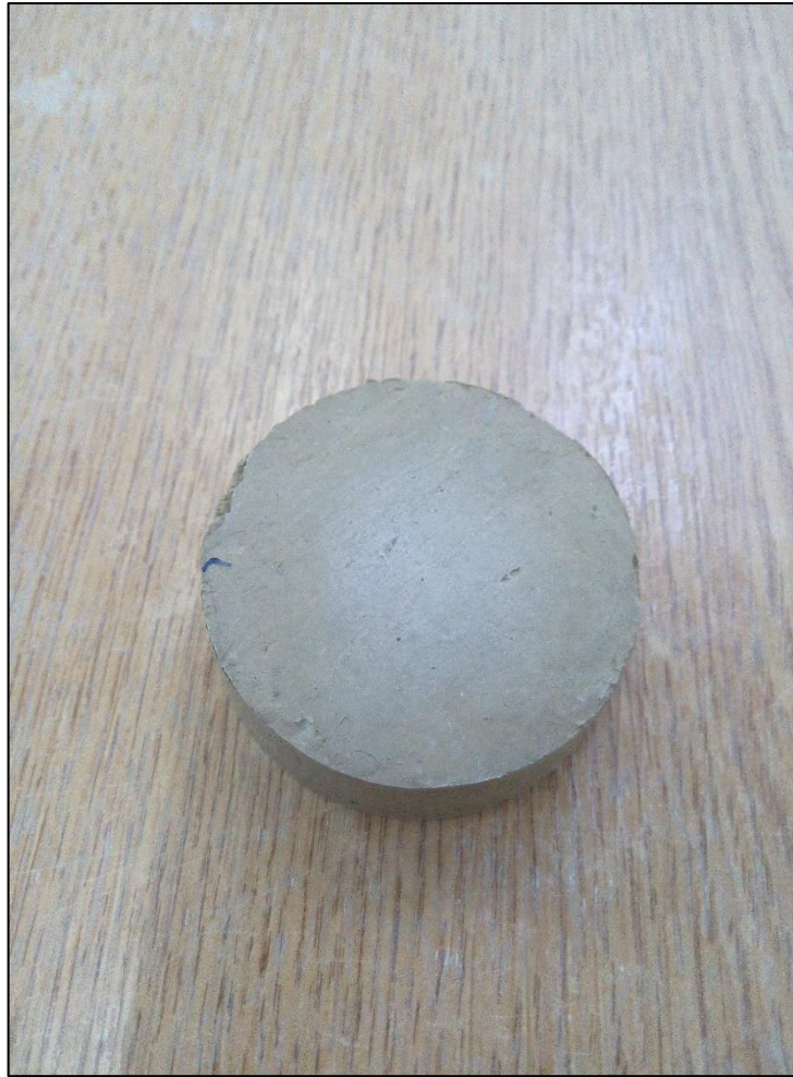
Figure A.29. Sample preparation of one dimensional consolidation test at 11% initial water content
