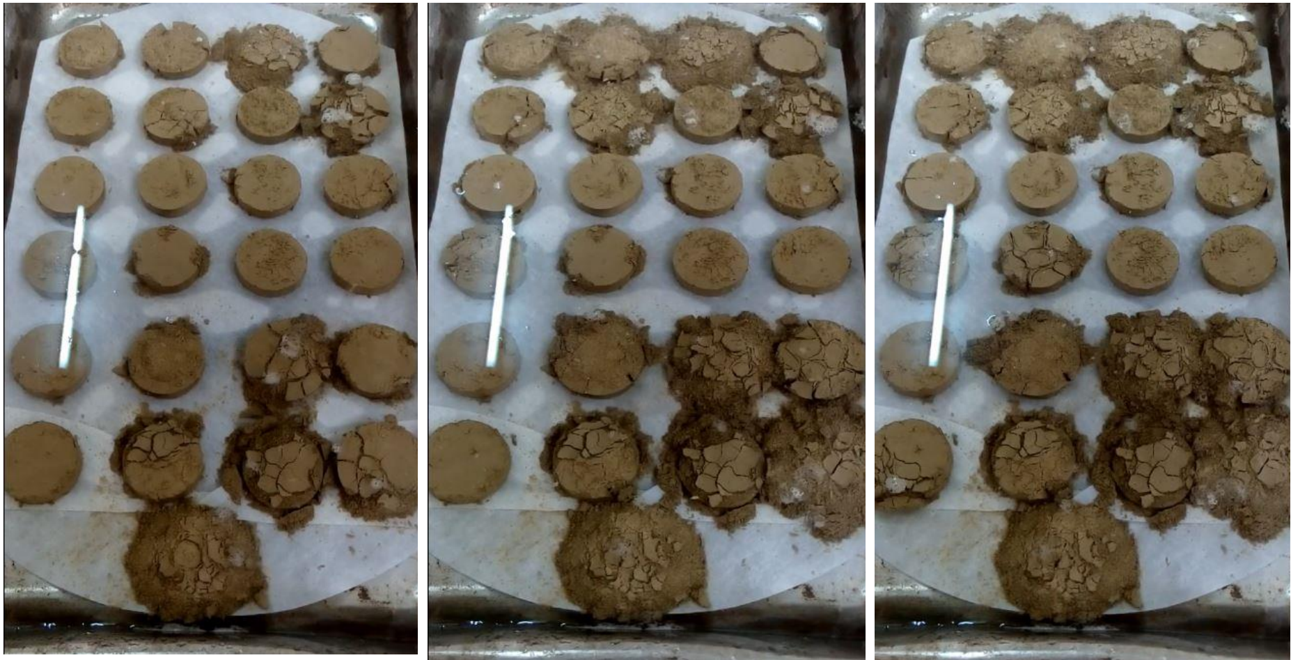
Figure A.14. Internal stability for untreated specimens with 16% initial water content at the end of a) 10 min, b) 20 min, C) 30 min
