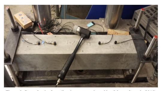
Figure 8: Setup for the free vibration test conducted by (Moustafa et al., 2015).
