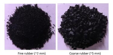
Figure 1: Fine and coarse rubber particles (Mousa, 2017)
