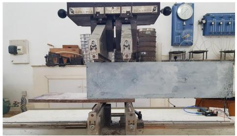
Figure 23: Setup of the free vibration test
