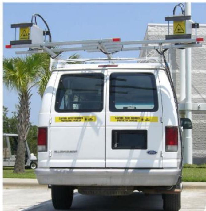
Figure 14: Laser-based vehicle for pavement data collection (Tsai & Li, 2012)
