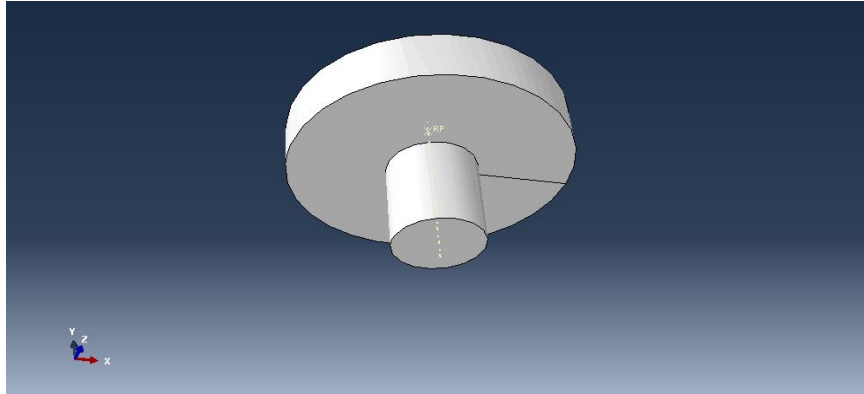
Figure 3.3: Simulation of tool shoulder and pin
