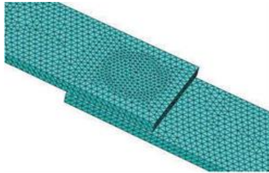
Figure 2.2: FE 10-node quadratic tetrahedron mesh [28]
