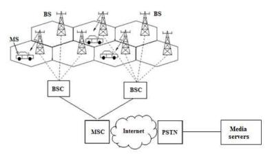
Figure 6: Architecture of a cellular wireless network
