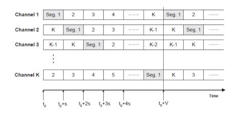
Figure 1: Broadcasting video segments in staggered broadcast manner [16]
