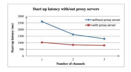
Figure 43: Effects off using proxy server in cellular networks
