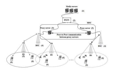
Figure 44: Peer-to-Peer communication based proxy server
