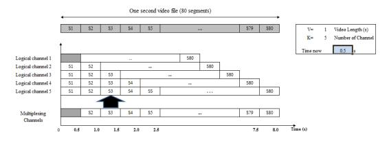
Figure 22: Multiplexing channel/multicast, time= 0.5 s
