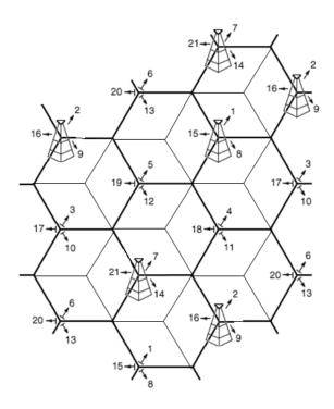
Figure 8: Multi frequency and frequency reuse based on sector antenna, where N=7
