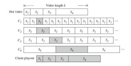
Figure 2: Illustration of segment downloading for the SkB technique, where number of channels is k=4, [19]
