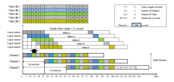
Figure 35: Multi-channel /multi-video implementation at time=100 s
