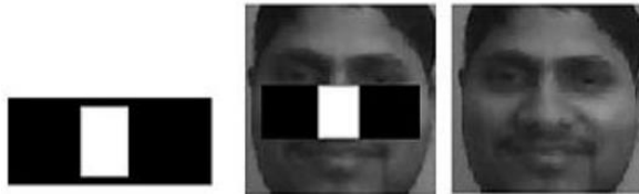
Figure 8: Haar Feature that looks similar to the bridge of the nose is applied onto the face
