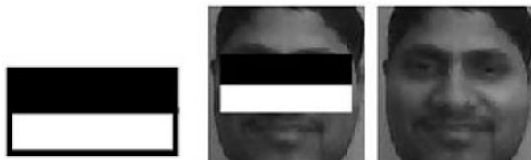
Figure 9: Haar Feature that looks similar to the eye region which is darker than the upper cheeks is applied onto a face.
