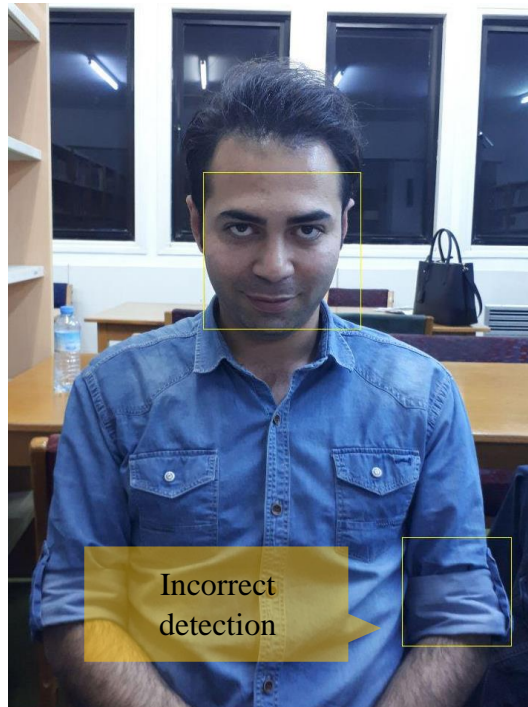
Figure 18: Sample of incorrect detection because of illumination noises
