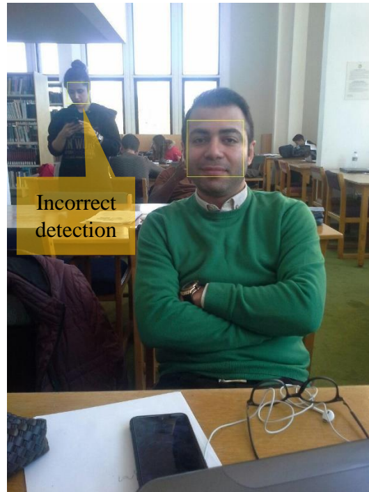
Figure 21: Example of crowded background which is cause of confusing the system
