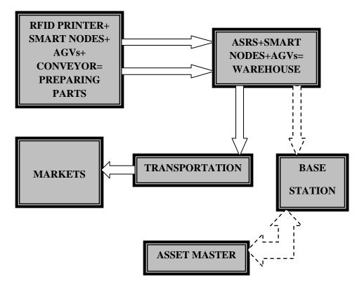
Figure 6.1: Structure of Introduced Intelligent Supply Chain
