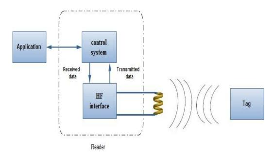
Figure 3.4: RFID Block Diagram Showing the Main Units
