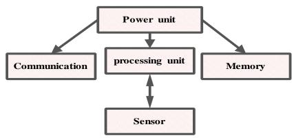
Figure 3.9: Parts of a Node
