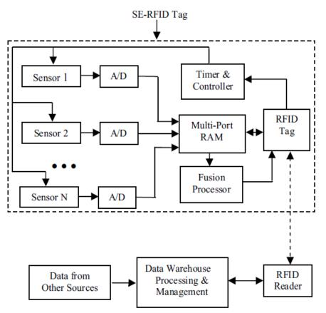
Figure 4.2: Sensor-Embedded RFID Type 1 [13]
