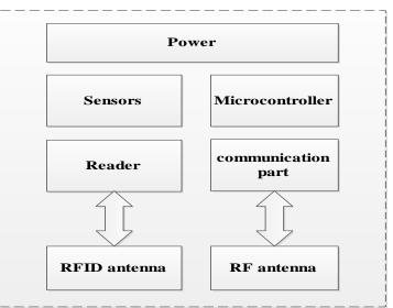
Figure 5.1: Components of Smart Node
