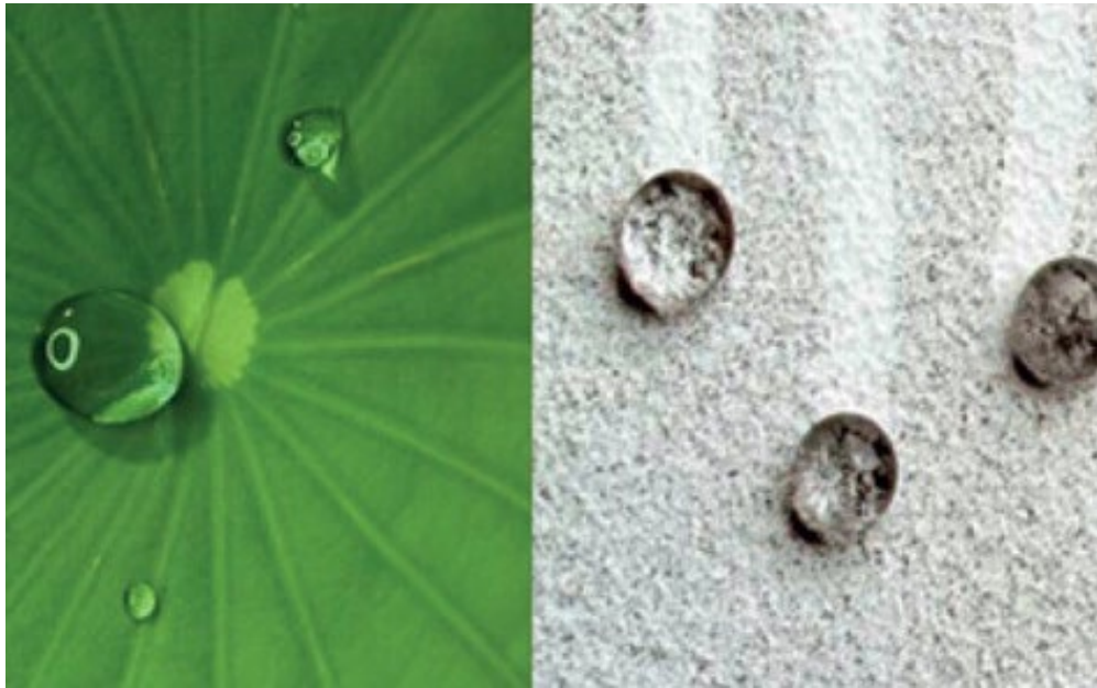
Figure 10: Lotus Plant Self-Cleansing Property, Biomimetic Design with Bottom-Top approach (Cuce, et al., 2019)
