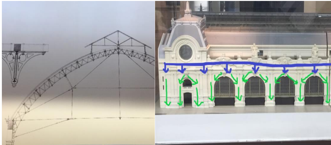
Figure 4.48: Arch construction and Exterior Load Path ( https://ceelondonblogs.ce.gatech.edu/blog_3 ) 2018
