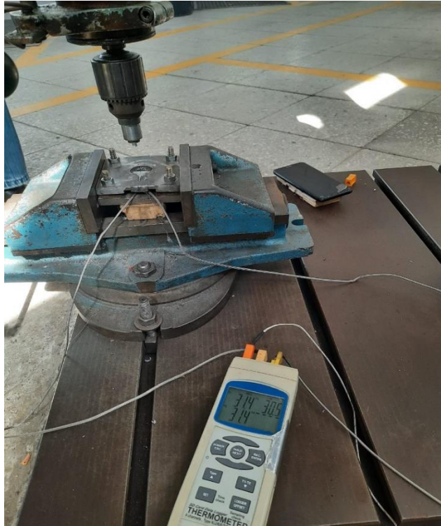
Figure 29: Temperature recorded of the weld joint with thermometer PCE-T390.
