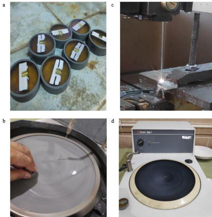
Figure 30: (a) Cold mount prepared samples, (b) EDM wire cutting machine, (c) Grinding process of samples, (d) Polishing machine
