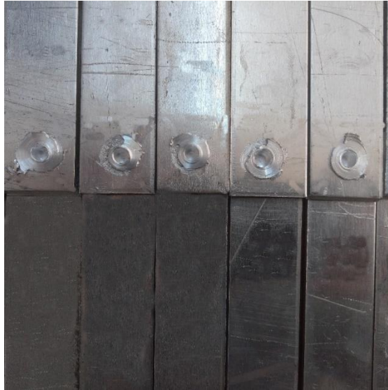
Figure 27: FSSW of AA5052 welded samples.
