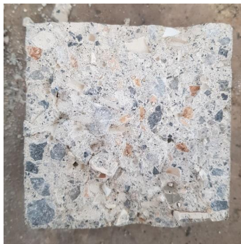
Figure 29: Splitted surface of concrete specimen after exposure to 200°C
