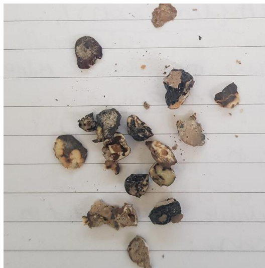
Figure 31: Damaged e-plastic particles after exposure to 300°C
