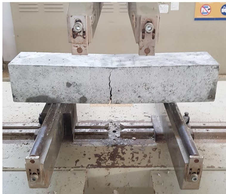
Figure 21: Concrete beam with inclusion of e-plastic aggregates in flexural strength test
