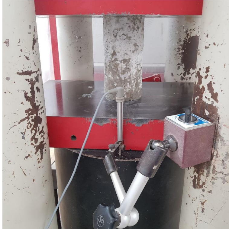
Figure 7: Load- deformation test under compression
