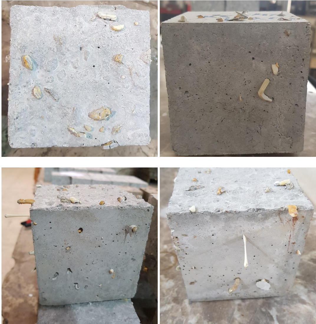
Figure 28: Surfaces of concrete specimens after exposure to 200°C
