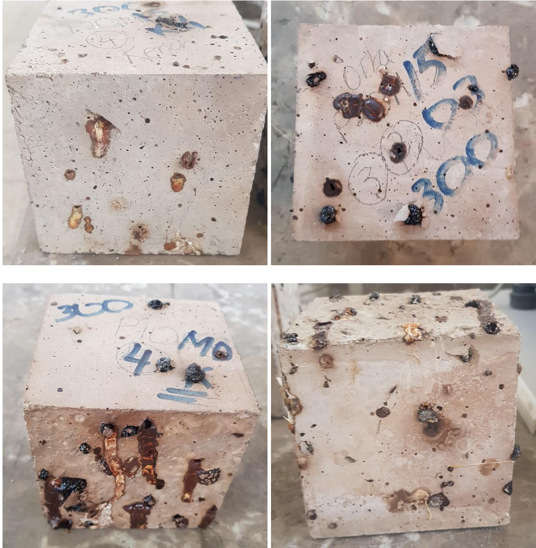
Figure 30: Surfaces of concrete specimens after exposure to 300°C
