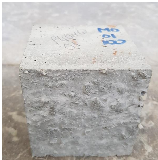
Figure 27: Surface of the concrete specimen after exposed to 100°C
