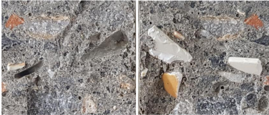
Figure 13: Concrete specimens with e-plastic after splitting tensile strength test
