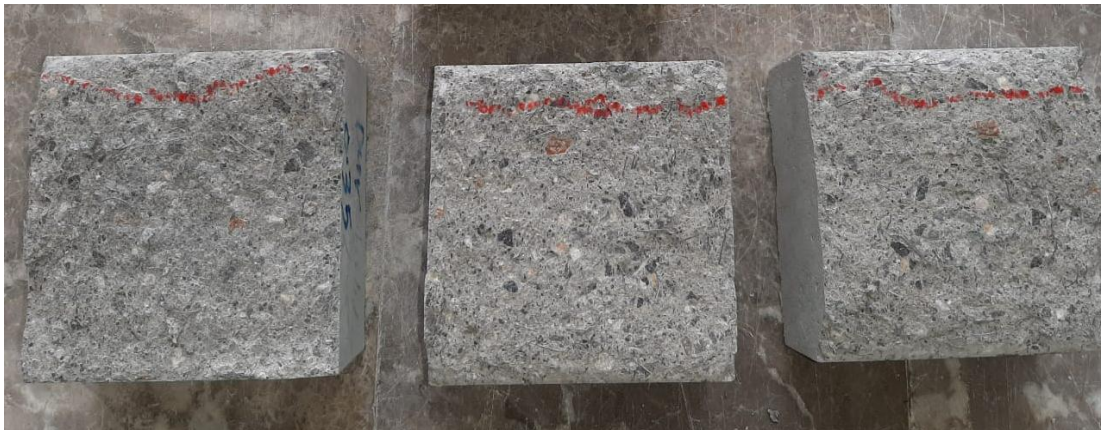
Figure 28: Effect of adding steel fiber on water penetration depth of SCC. (a) 0.35%, (b) 0.45%, (c) 0.55% volume fractions
