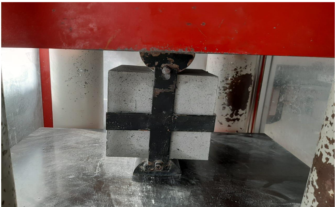
Figure 14: Splitting the samples to measure water penetration depth
