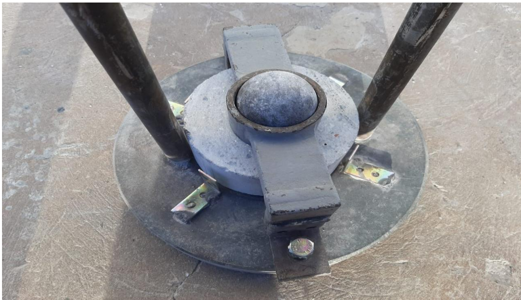
Figure 11: Impact resistance test of the sample
