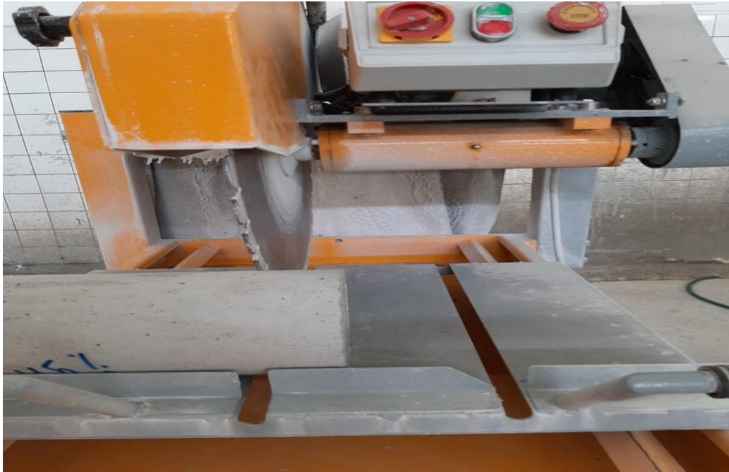
Figure 10: Cutting machine used to prepare impact test samples
