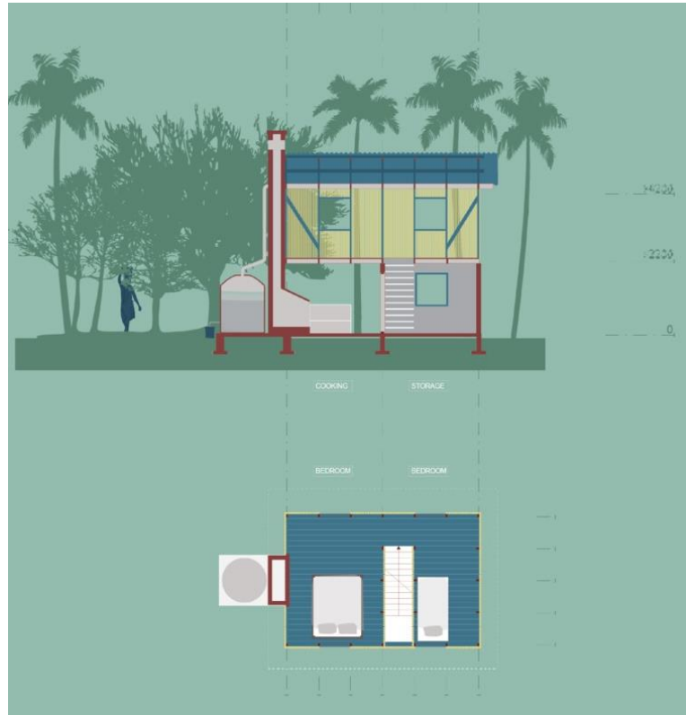
Figure 22: First Floor Plan and Section of Magoda Project Case Study
